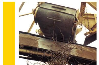
What's more, pole plates are integrated in the housing to concentrate the magnetic flux. Along with the electromagnetic coils, the cross-section, structure, shape and size are responsible for STEINERT electromagnets excellent sorting capability. The result is that the electric suspension magnet is extremely effective despite its compact size, low weight and low power consumption. STEINERT consistently uses air-cooled, "dry" electro suspension magnets without oil filling.
