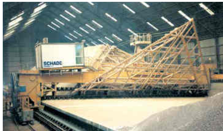
Bridge Scraper Reclaimer, 26.4 m span, 250 t/h, Limestone
