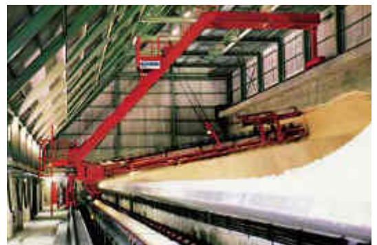
Semi-Portal Scraper Reclaimer, 14 m span, 80 t/h, FGD-Gypsum
