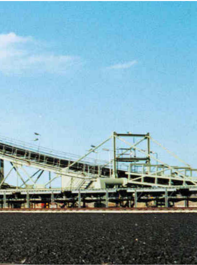
Fig. 2 Slewing/Luffing Stacker for 1,000 t/h Coal
