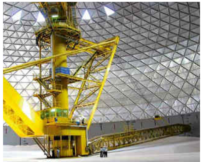
Cantilever Scraper Reclaimer, dia 120 m, stacking 2,500, reclaiming 250 t/h, Salt
