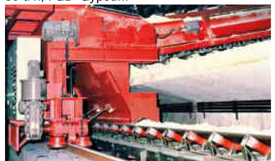
Direct discharge on belt conveyor
