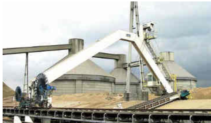
Portal Scraper Reclaimer, 33 m span, 600 t/h, Slag
