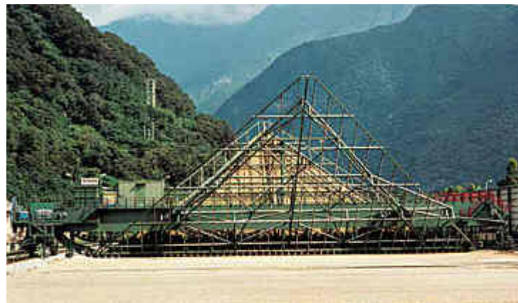
Bridge Scraper Reclaimer, 56 m span, 1.200 t/h, Limestone
