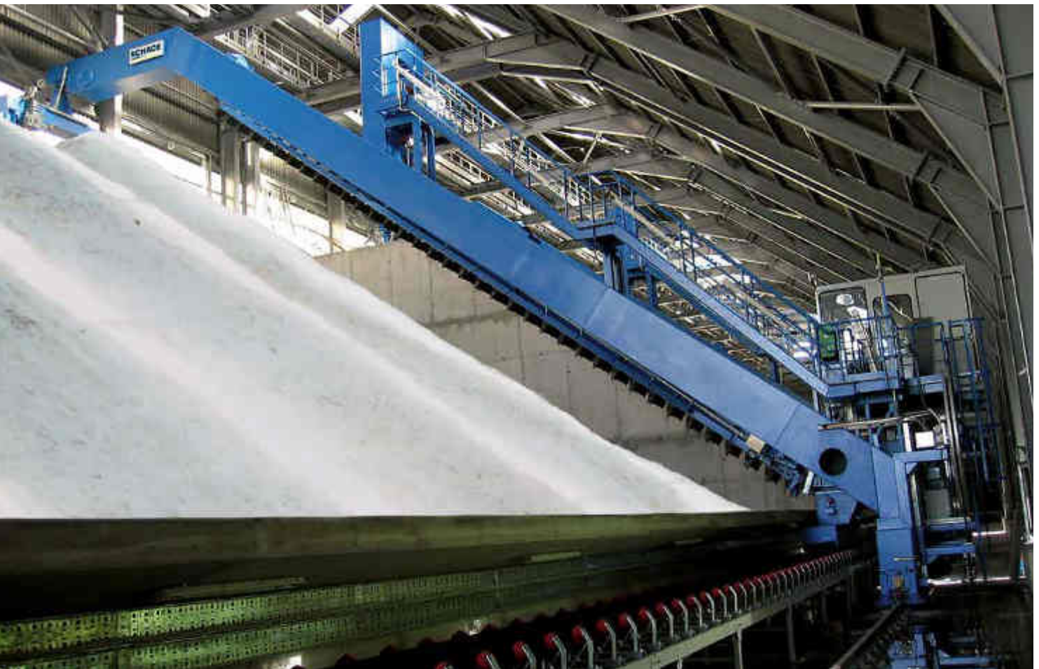
Semi-Portal Scraper Reclaimer, 21 m span, 150 t/h, additives
