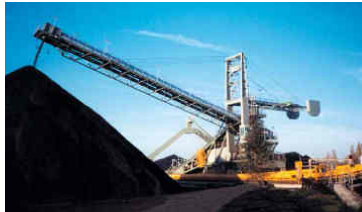
Fig. 2 Slewing/Luffing Stacker for 1,000 t/h Coal
