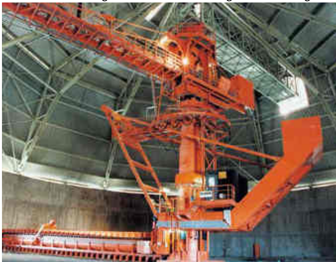
Circular Stacker / Cantilever Scraper Reclaimer, dia 61 m, stacking 1,700 t/h, reclaiming 2,500 t/h, Iron Ore concentrate
