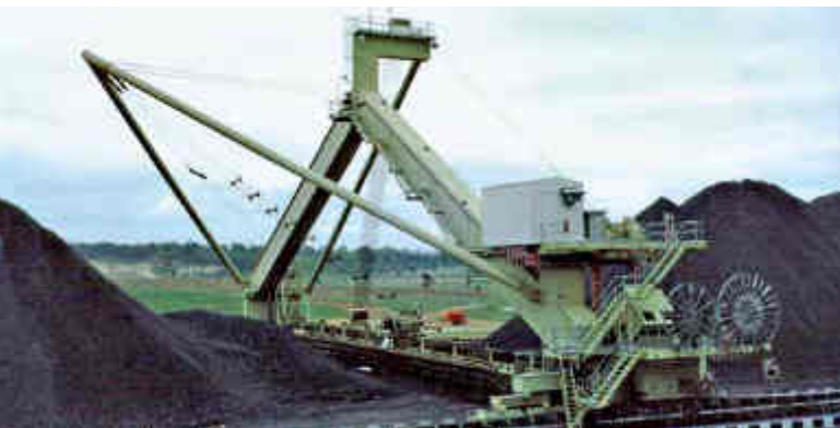
Portal Bridge Reclaimer, 50 m span, 600 t/h, Coal
