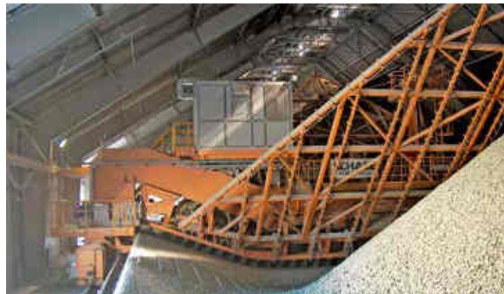
Bridge Scraper Reclaimer, 27.5 m span, 300 t/h, Gypsum
