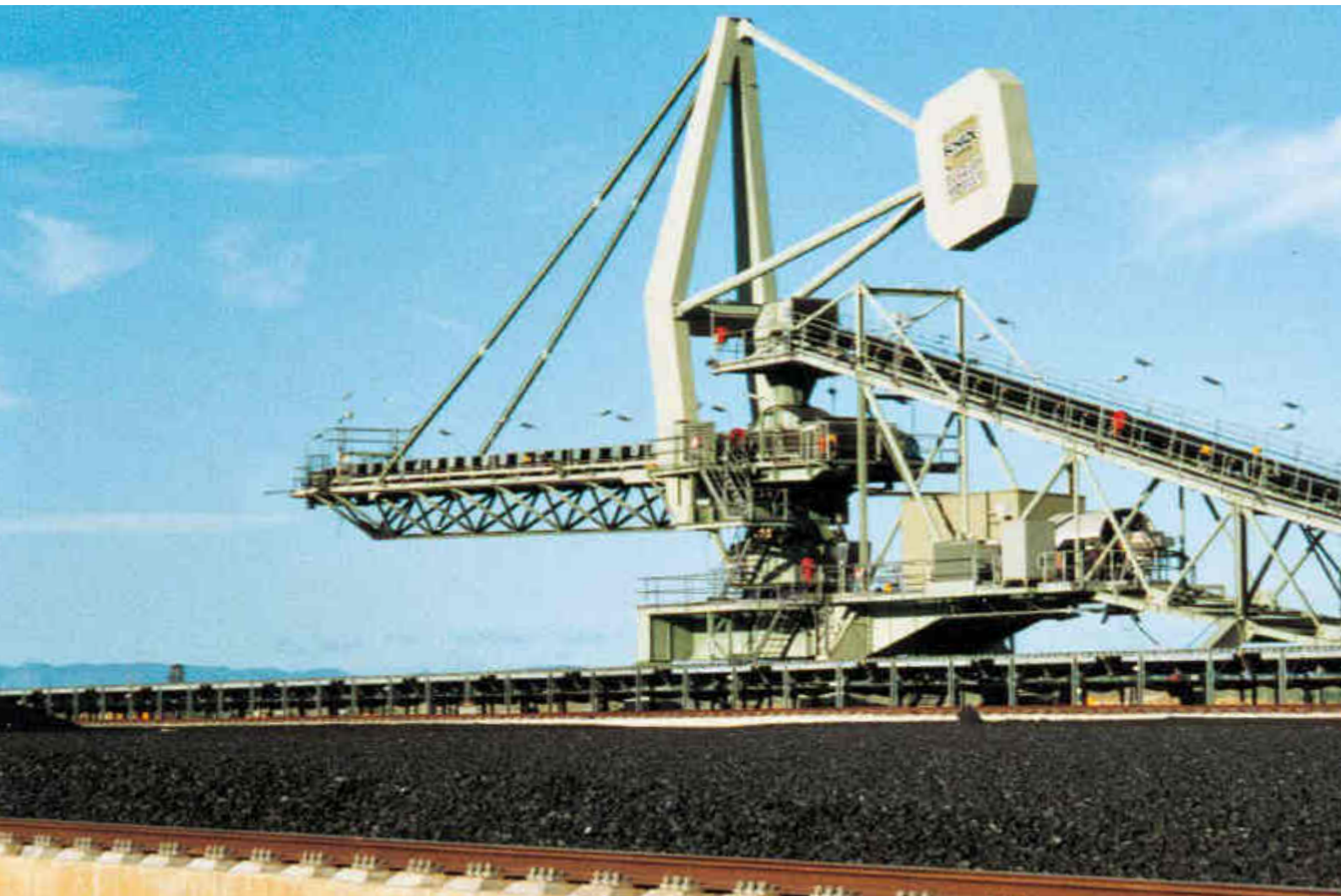
Fig. 1 Slewing/Luffing/Stacker for 2,750 t/h Coal
