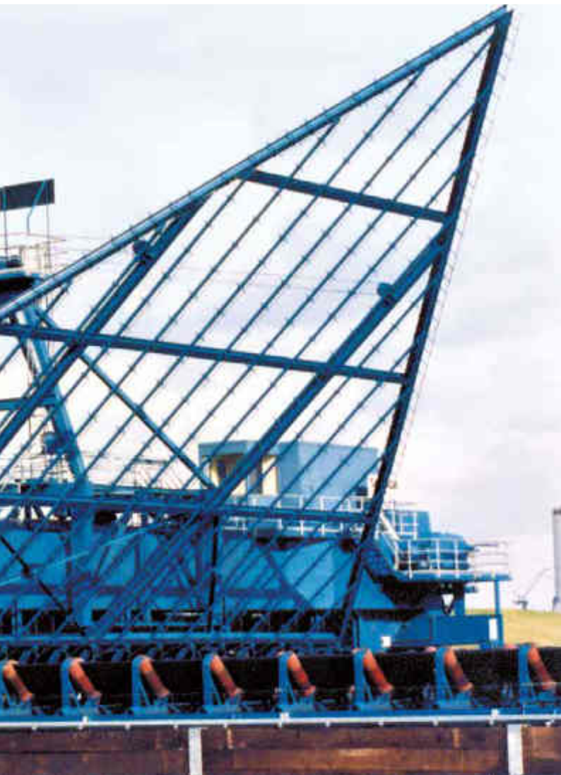
Bridge Scraper Reclaimer, 26.4 m span, 250 t/h, Limestone
