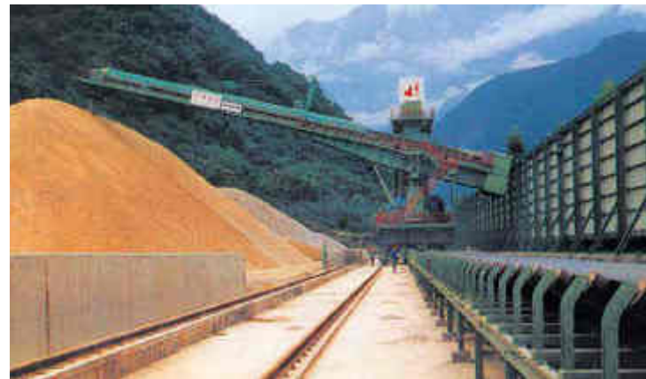
Fig. 3 Luffing Stacker for 2,000 t/h Limestone
