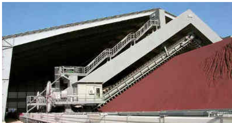
Portal Scraper Reclaimer, 49 m span, 550 t/h, additives
