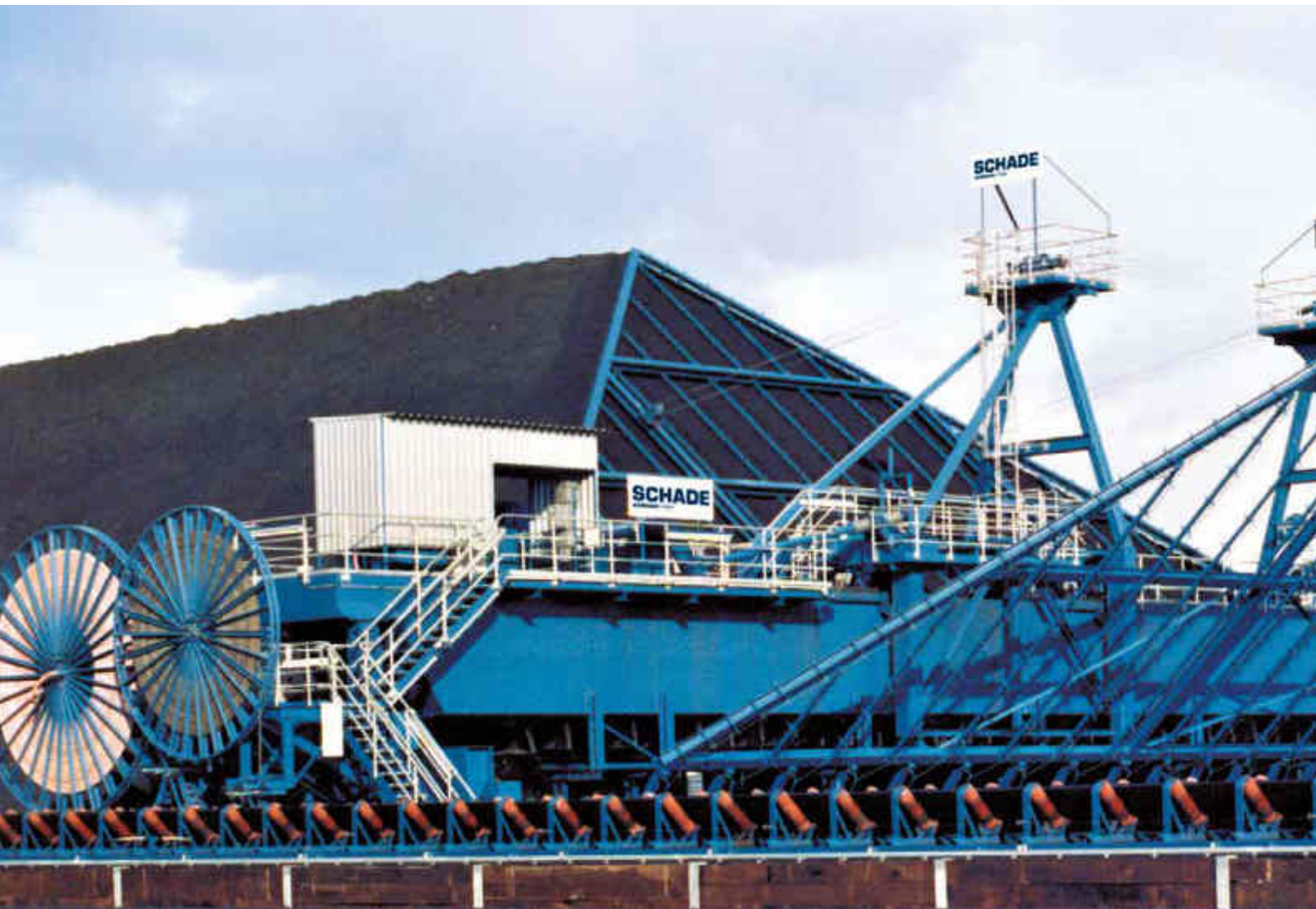
Bridge Scraper Reclaimer, 50 m span, 1,100 t/h, Coal
