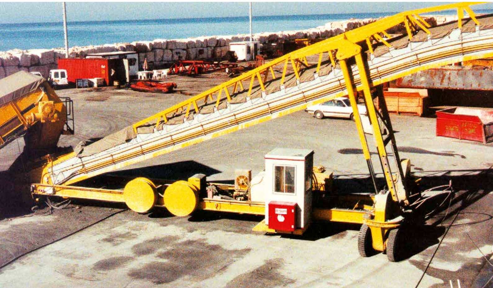
Powered radial operation with in-line tow travel
