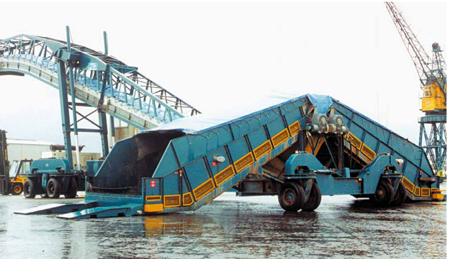
Twin Samson® Material Feeders with flexible enclosures
