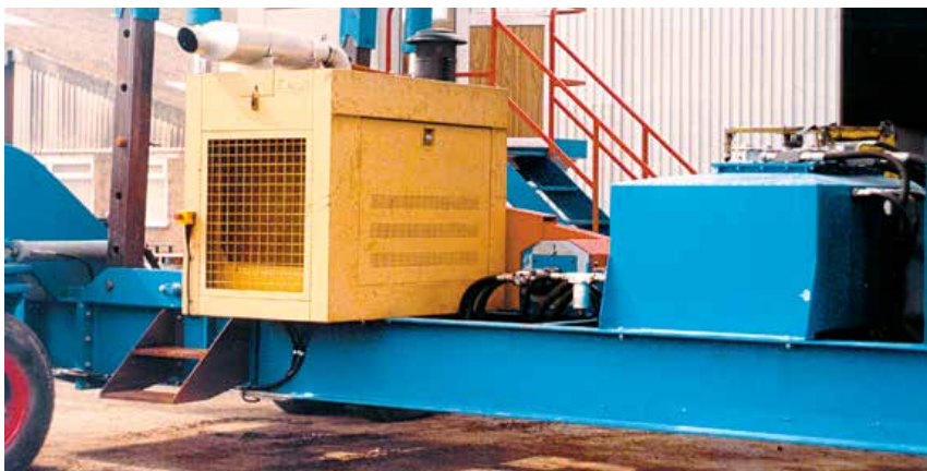
Auxiliary Gen-Set drives the powered travel system only
