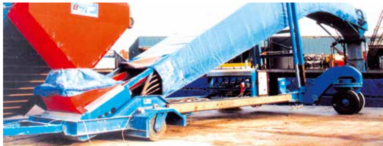
Tail end castor-wheel mounts with parallel push travel
