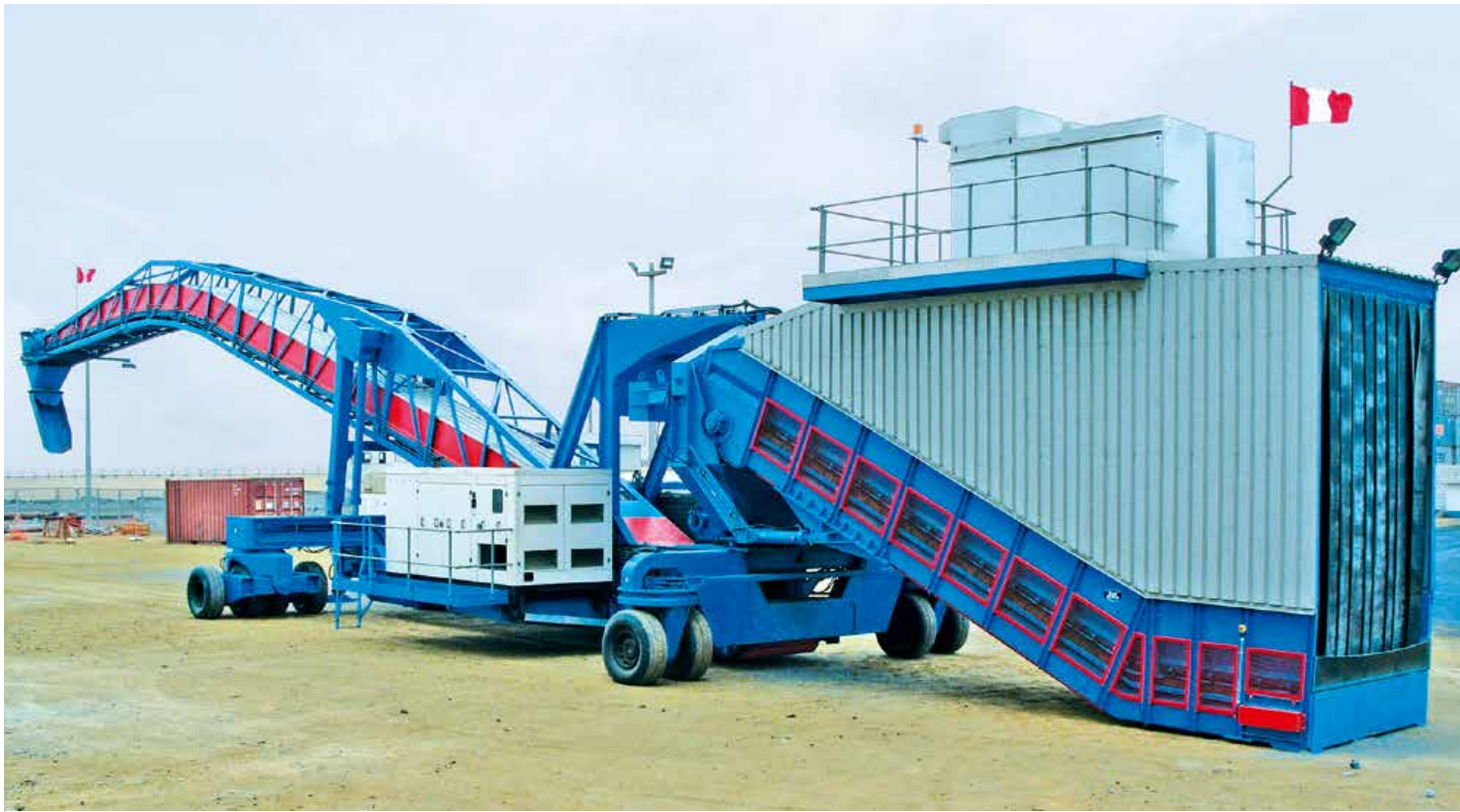
Samson® Material Feeder mounted on slewing frame to Shiploader chassis
