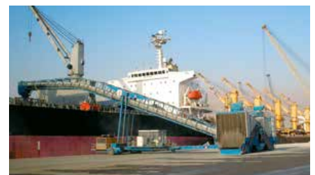
Shiploader with Twin Samson® Material Feeders loading Panamax vessel
