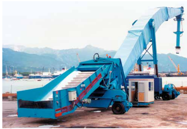
Samson® Material Feeder raised for travelling
