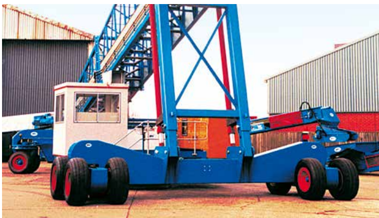
Forward axle beam with telescopic boom supports
