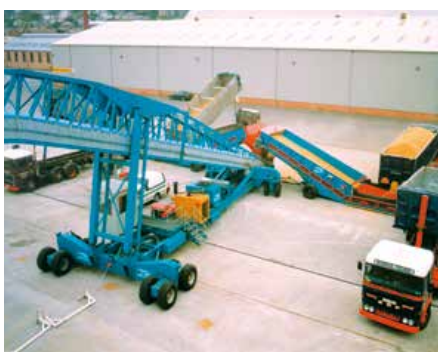
Twin independent multi-feed-point Samson® Material Feeders discharge to a single Shiploader
