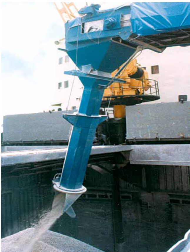
Two stage variable angle and telescopic trimming chute
