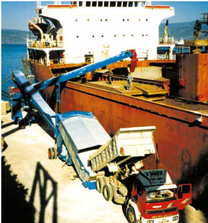
Raised chassis Shiploader with Stormajor® Feeder
