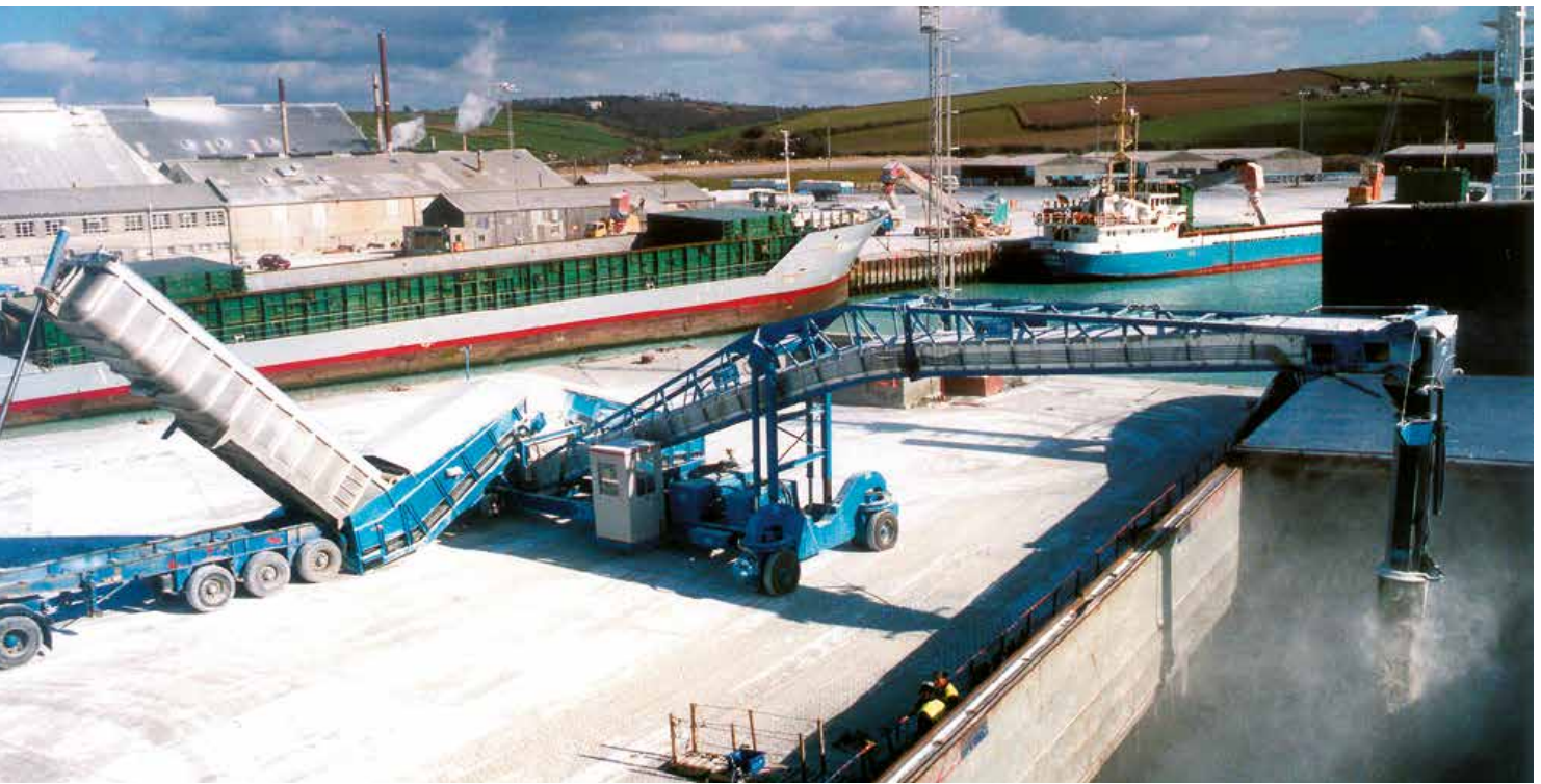
Twin integral Samson® Material Feeders mounted to the Shiploader chassis
