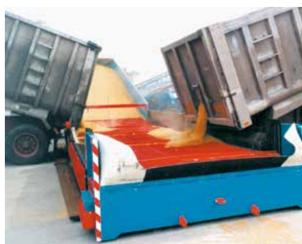
Up to four trucks discharge simultaneously per Samson® Material Feeder
