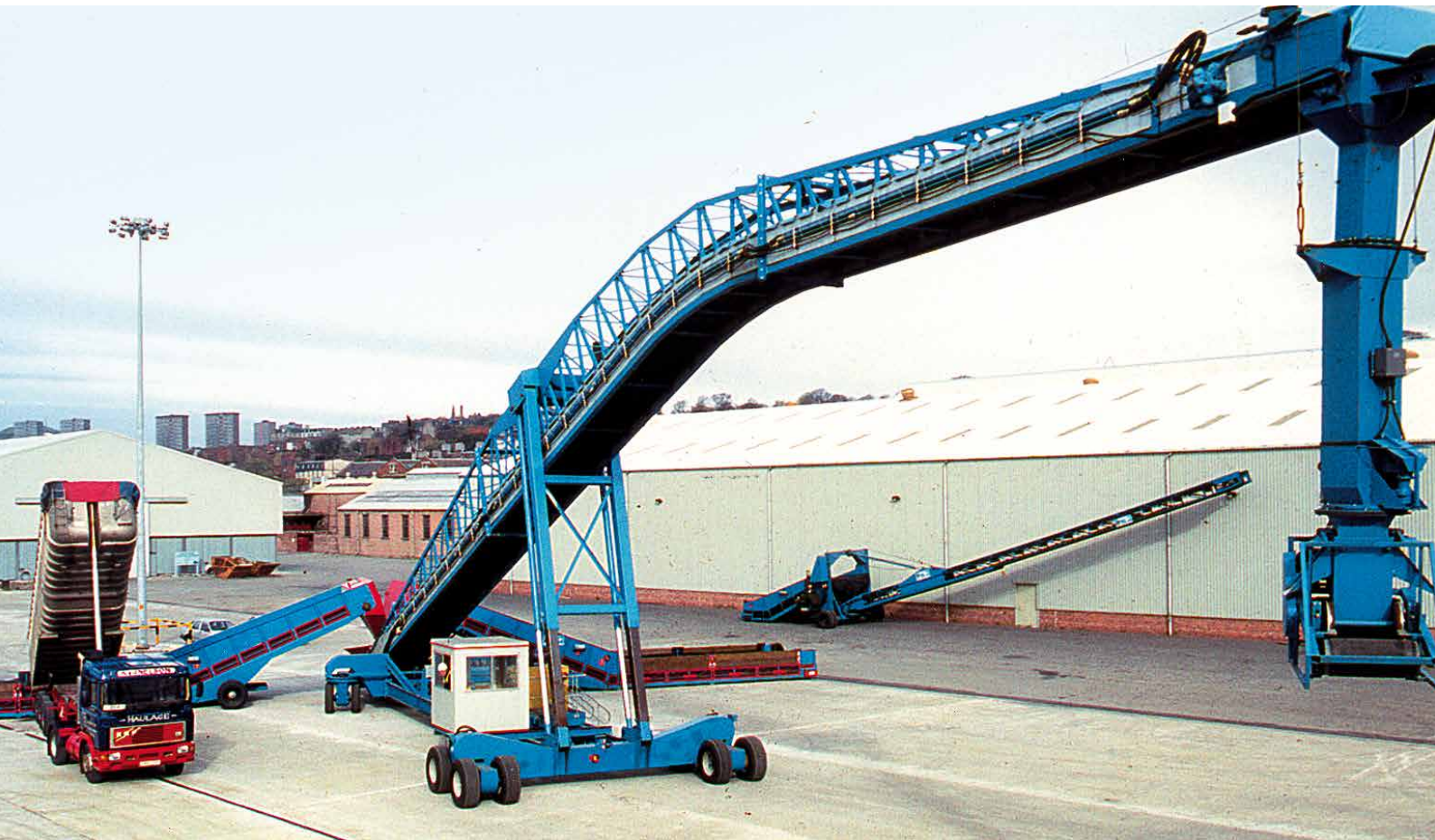
In-line powered travel with rear steering axles and twin tandem front axle
