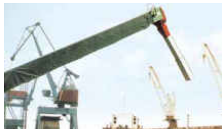
Extended trimming chute showing also the full boom enclosure using flexible PVC covers
