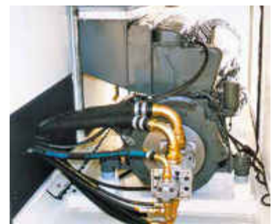
Diesel motor drive with triple section hydraulic pump system fitted to the side of the main chassis within a sound attenuated enclosure
