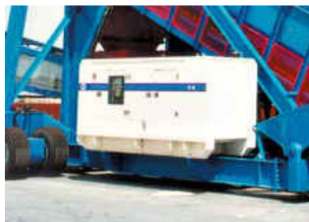
Diesel Gen-Set mounted to the main chassis within a sound attenuated enclosure
