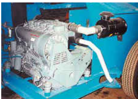
Deutz diesel motor with direct coupled hydraulic drive mounted beneath the Samson® inclined section
