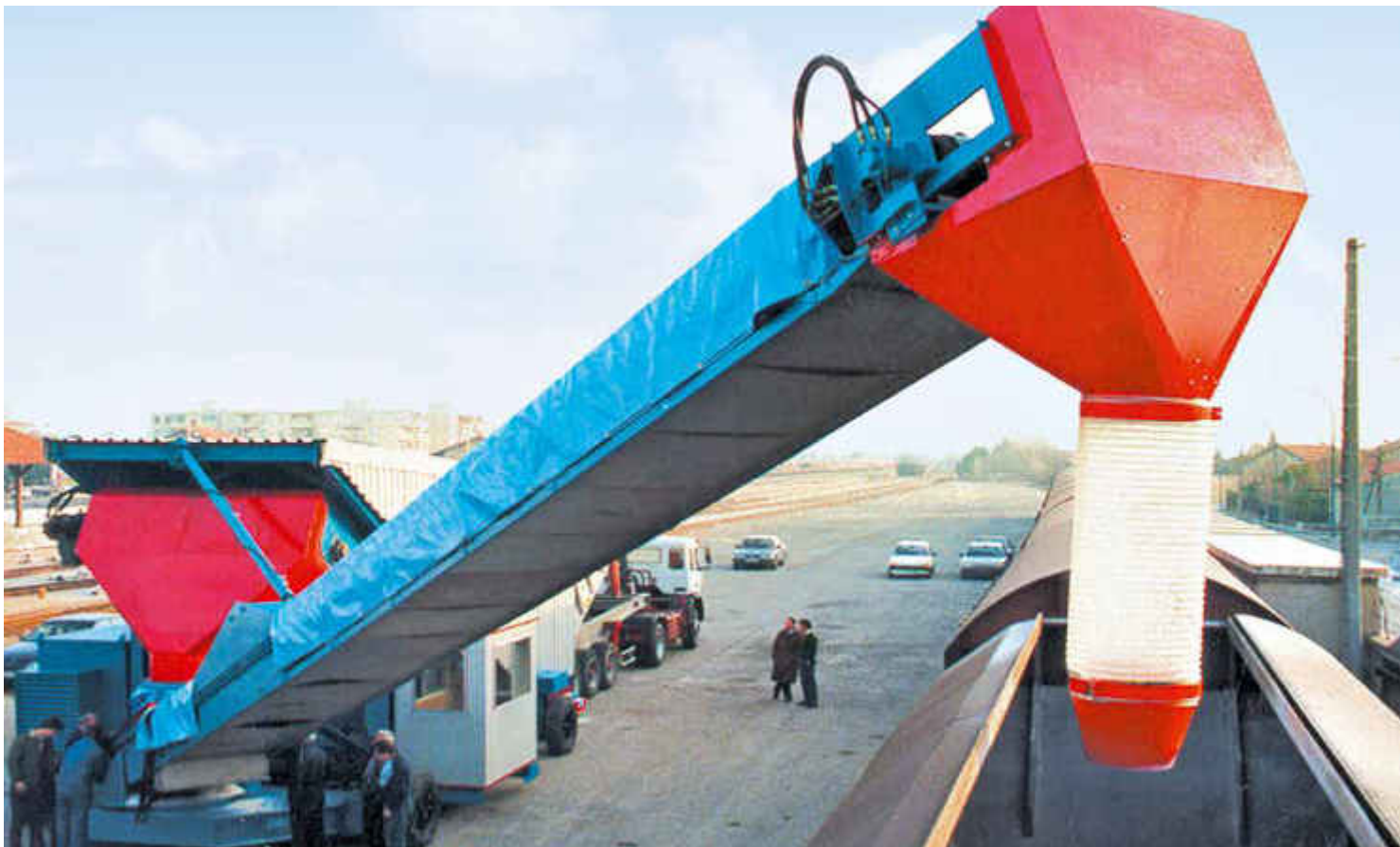
Outloading boom with hydraulic head shaft drive shown here with full enclosure system - loading sand to rail wagons
