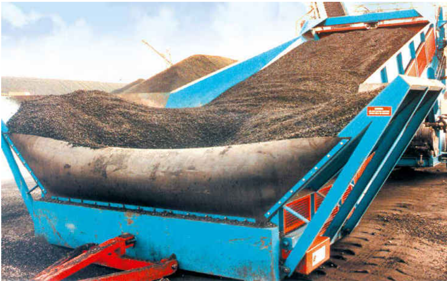
Stormajor® receives coal from loading shovel for stockpiling and barge loading
