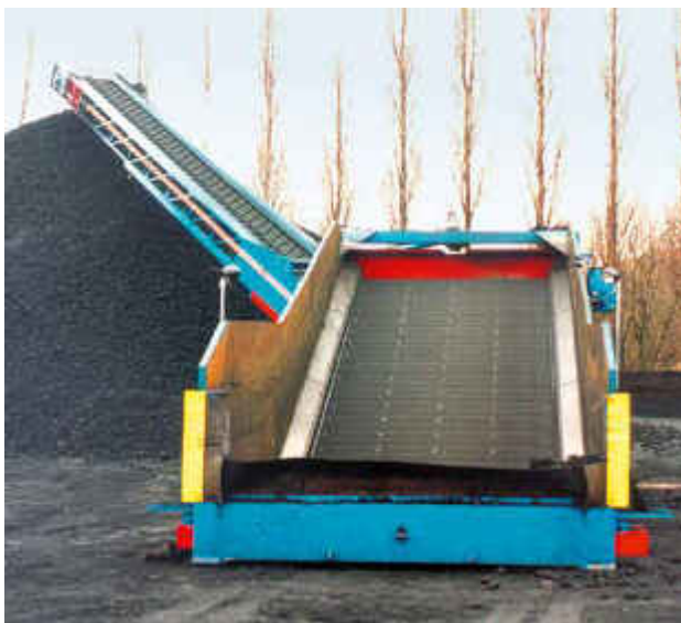
Stormajor® handling smokeless fuel briquettes direct from tipping trucks
