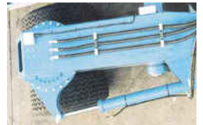
Hydraulic Actuator Steering System with slewing ring mounting for the twin wheel units.
