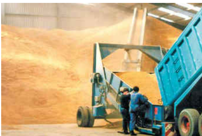
Stormmajor® loading cereals to covered flat storage
