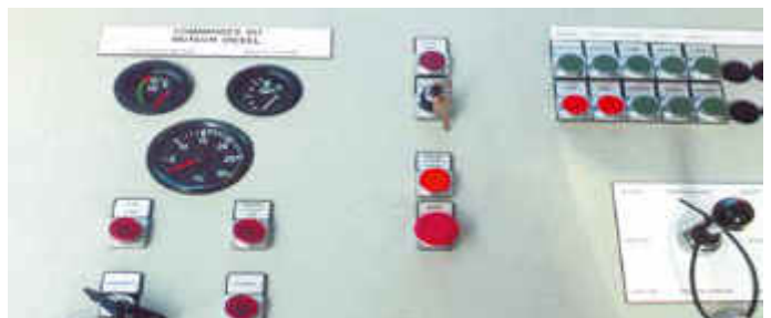
Comprehensive control panel with integral diesel motor instrumentation and joy stick controller for powered travel system operation
