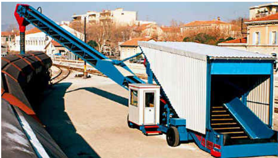
Stormajor® handling silica sand from tipping trucks to rail wagons
