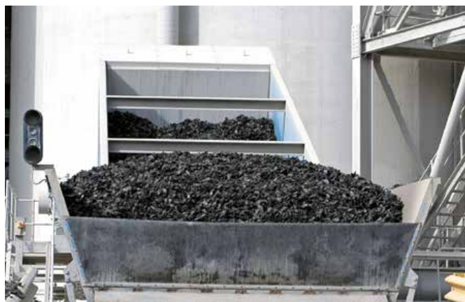
The Samson® Material Feeder supplied with a screw metering feeder across the discharge to meter the tyre chips to a vertical bucket elevator discharging to a high level bunker
