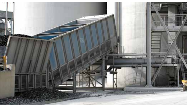
The Samson® Material Feeder supplied with a screw metering feeder across the discharge to meter the tyre chips to a vertical bucket elevator discharging to a high level bunker
