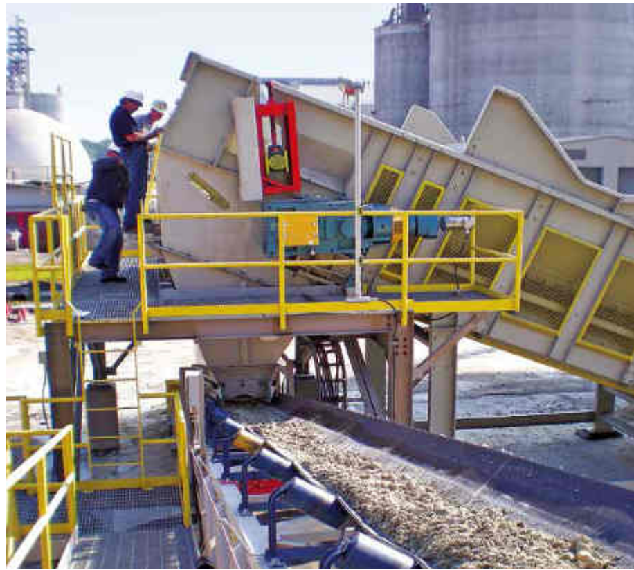
Samson® Material Feeder MF16xxx with tandem drives using two helical/bevel speed reducers mounted one each side of the extended head shaft
