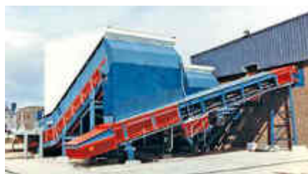
The Samson® Material Feeder horizontal storage bunker with overhead conveyor and plough discharger
