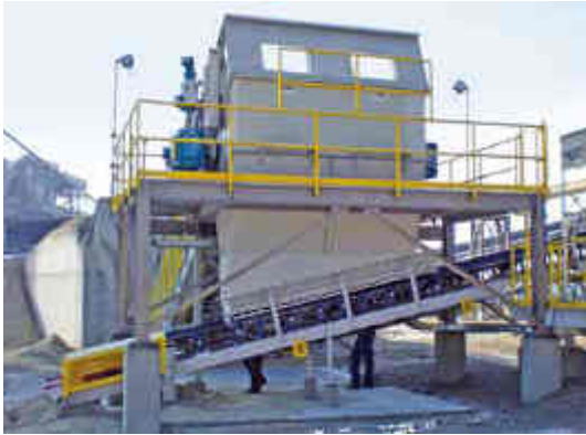
Samson® Material Feeder MF16xxx with tandem drives using two helical/bevel speed reducers mounted one each side of the extended head shaft
