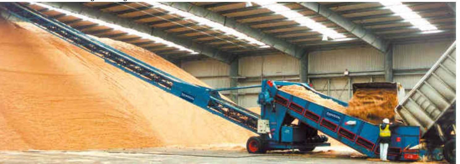
Stormajor® combines the benefits of a Samson® Material Feeder with a radial stacking boom mounted to a common mobile chassis
