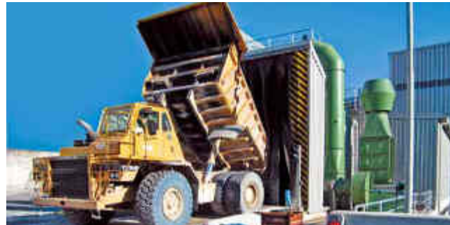
Enclosure with extended flared entry for large mining dump trucks
