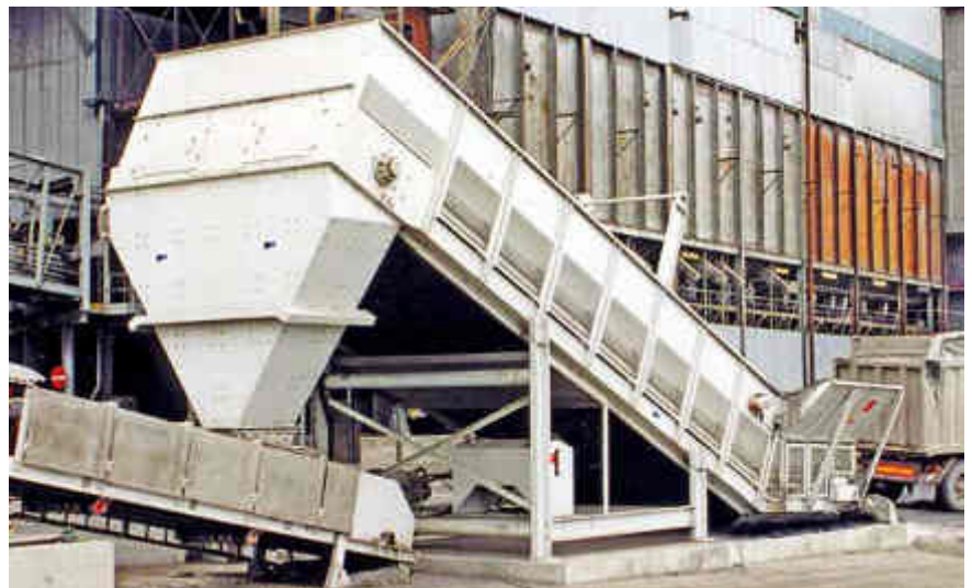
The Samson® Material Feeder with a centralising head chute discharges to a conveyor positioned in-line
