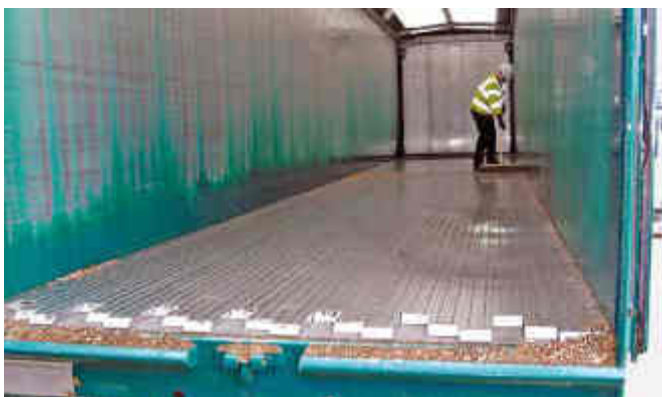
Intake from high capacity live floor trailers
