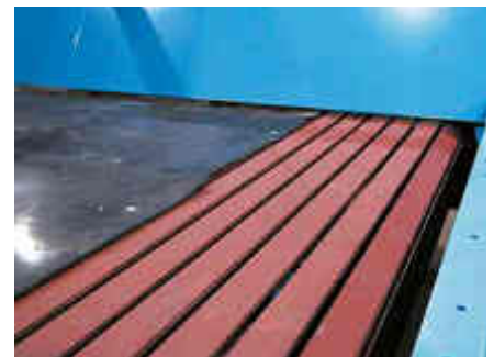
Steel apron bars support the load
