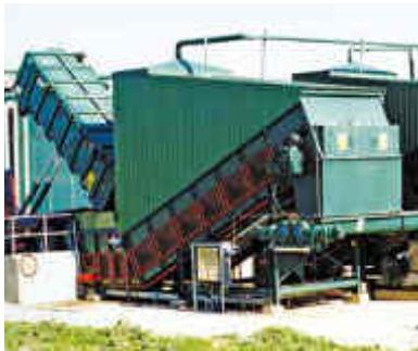
Enclosure with fume extraction for odious materials
