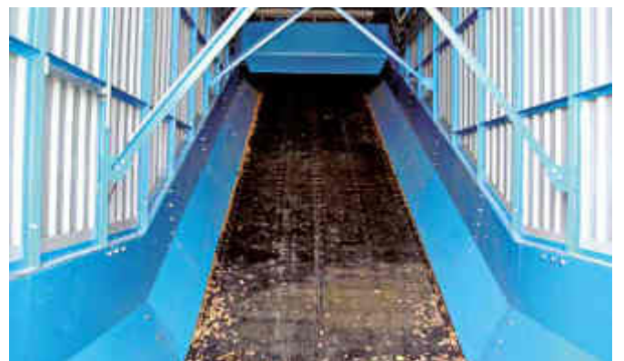
The wide apron-belt Samson® Material Feeder concept is ideal for difficult materials
