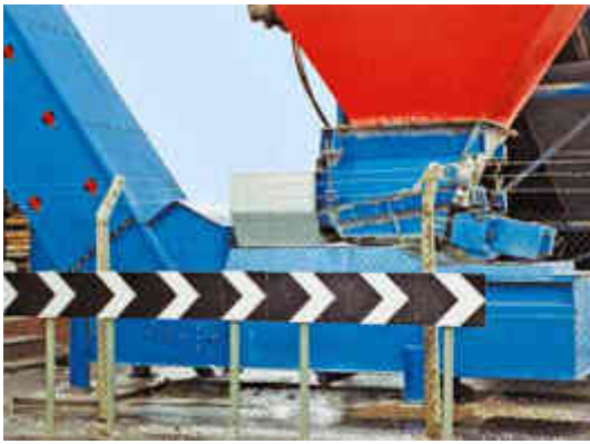
Vibro-Feeder controlling feed rate to a steep angle belt conveyor
