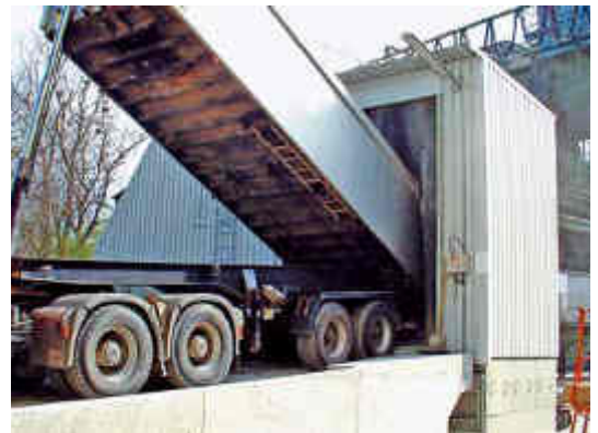
The side loading Samson® Material Feeder receives cement clinker for import directly to an existing conveyor installation
