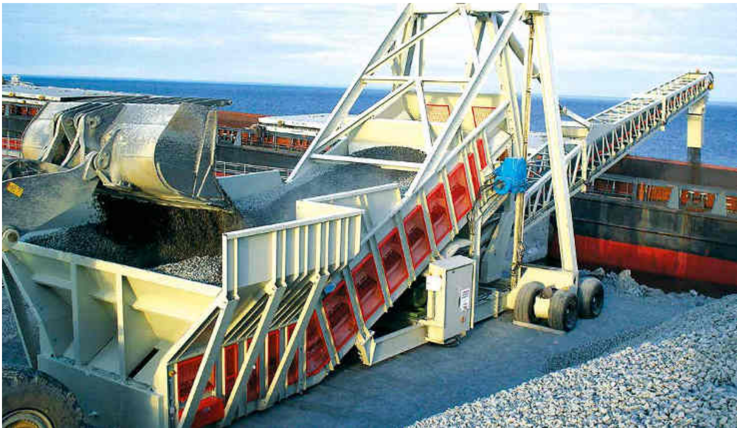
The massive Samson® Material Feeder MF16xxx receives gabbros rock from shovels for barge loading at 1,000 t.p.h.
