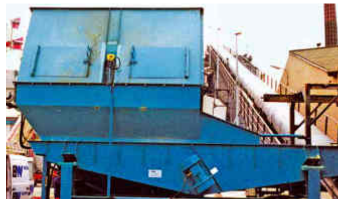
Vibratory feeder provides regulated output to an inclined belt conveyor
