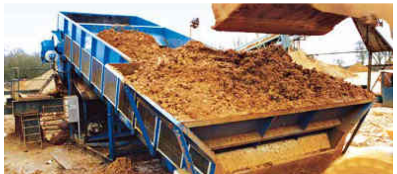
The Samson® Material Feeder with straight chassis and flared entry (width 4.5 m) receives sandy clay from shovels
