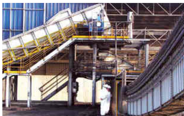
Samson® Material Feeder supplied with vibrating screen to remove oversize material before onward conveying
