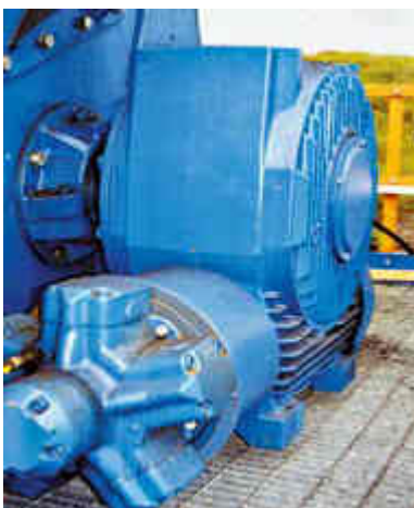
High efficiency helical/bevel main reduction gear with helical primary
