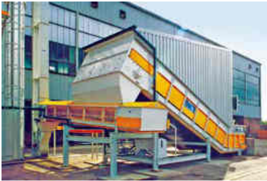
Kleen-line belt feeder transfer to Bucket Elevator
