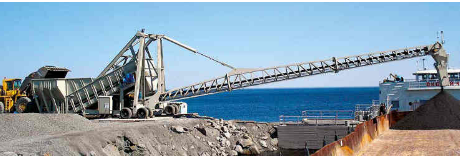
Stormajor® Radial Boom Stacker with integrated Samson® Material Feeder MF16xxx series and radial stacking boom for barge loading
