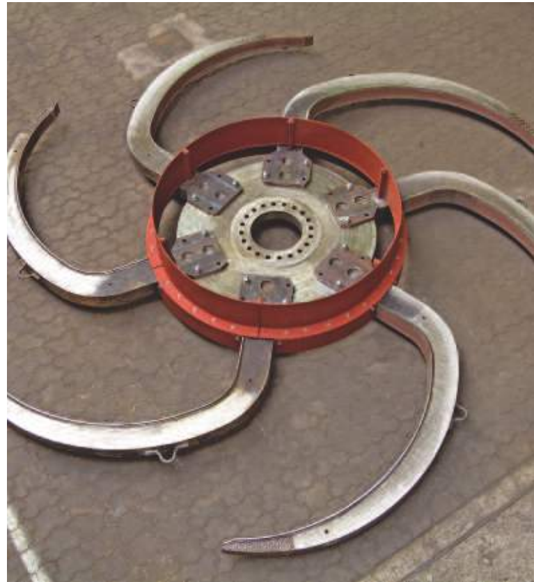
BEW-K discharge wheel, \varnothing 4,500 mm
