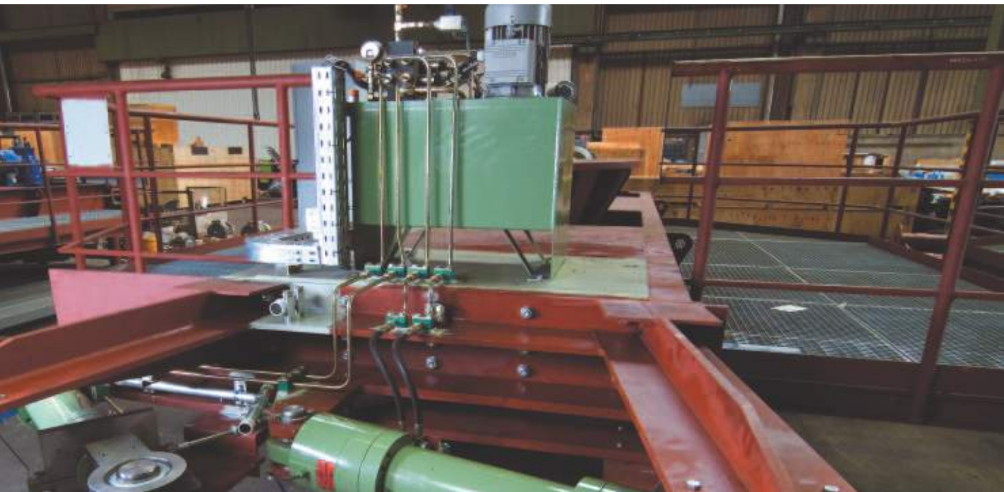
Chassis of BEW-K, view onto hydraulic cylinders for rotation
