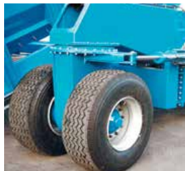
Twin Axle Steering Bogie with potentiometer alignment system to achieve Ackerman steering without a mechanical linkage.
