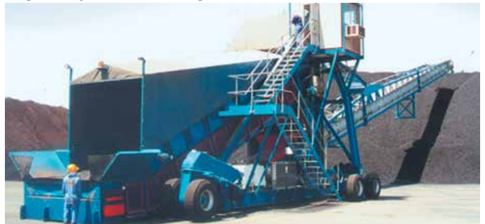
Control cabins may be mounted at high level as shown above or at low level on the main chassis
