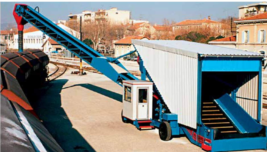
Stormmajor™ handling Silica Sand from tipping trucks to rail wagons
