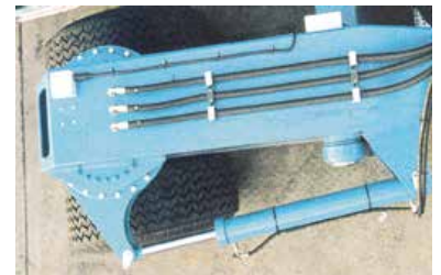
Hydraulic Actuator Steering System with slew ring mounting for the twin wheel units.
