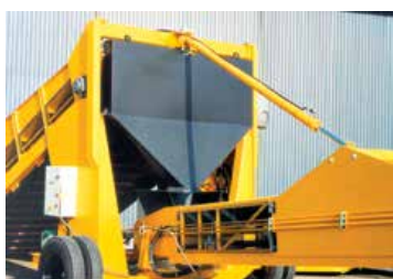
Stormmajor™ handling smokeless fuel briquettes direct from tipping trucks
