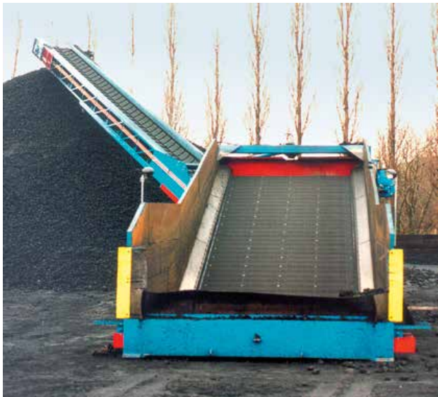
Stormmajor™ handling smokeless fuel briquettes direct from tipping trucks
