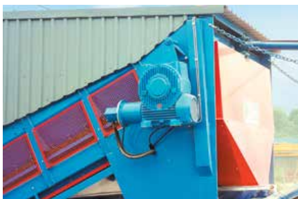
Drive to the Samson™ receiving section by direct coupled hydraulic motor with a shaft mounted worm reduction gear
