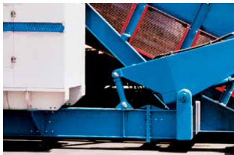
Jacking Axle shown here with the Samson™ lowered to ground level in the normal working position
