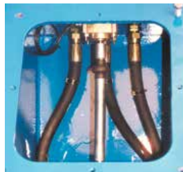
Rotary Potentiometer linked to the slew ring determines the wheel orientation and maintains both steering wheels in correct alignment using an electronic comparator system.
