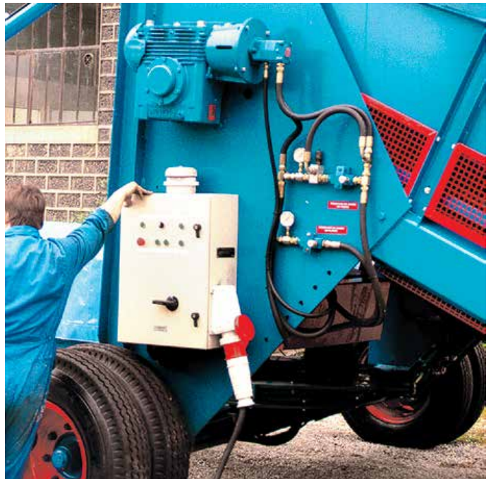
External control panel for electric motor drive with detachable cable
