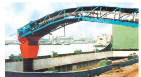
Extended Trimming chute showing also the full boom enclosure using flexible PVC covers
