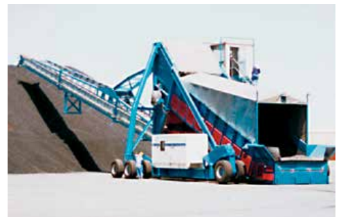
Jacking Axle shown here raises the Samson™ clear of the ground for travelling
