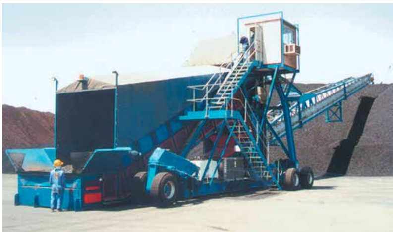
Material stored within the Samson™ body may be at various load levels along the length of the Samson™
