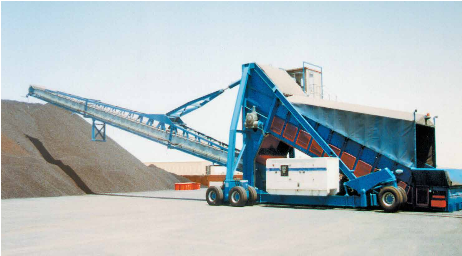
Stormmajor™ stockpiling various materials from wood chip to iron ore for a Middle East steel works stockyard
