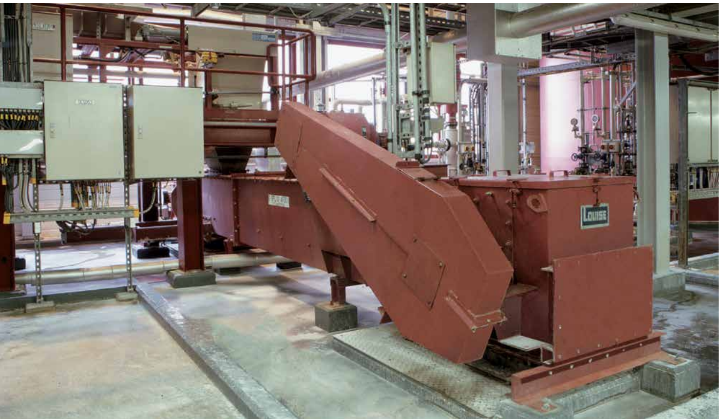
LOUISE Double-Strand Chain Conveyor feeding 2 silos
