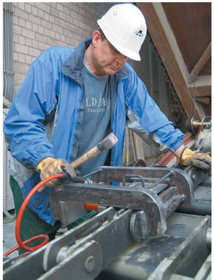
Pre-assembly of chain strands
