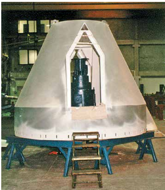
Ready assembled CTX-I 5000, view into the support/maintenance arm, onto the planetary drive unit
