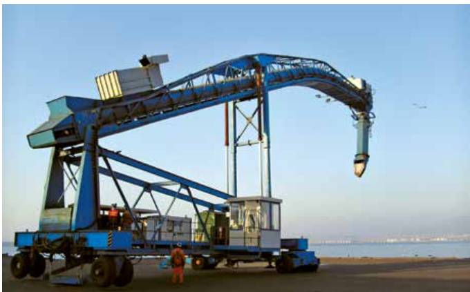
Raised chassis shiploaders available for Panamax ships
