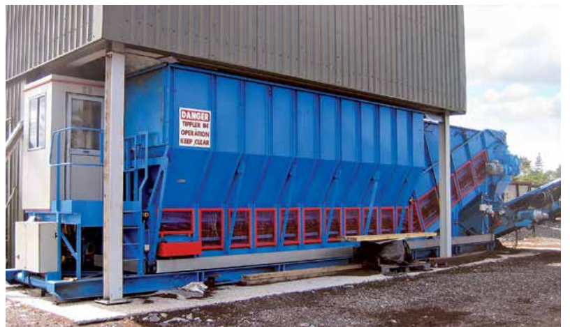
Skid Mount Box Feeder Receives from Wagon Tippler
