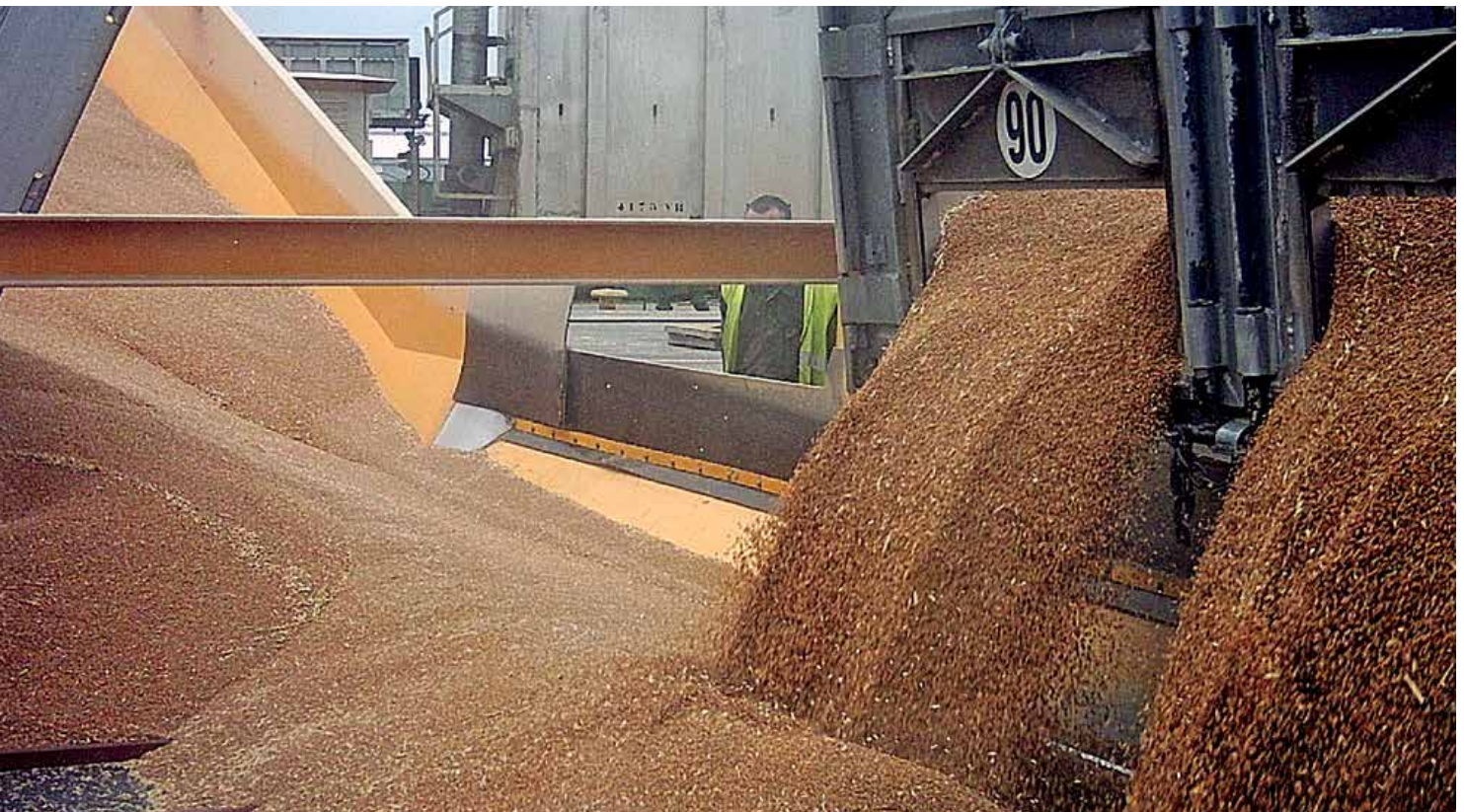
Independent Multi-Tip Samson™ Material Feeder with extended entry section to permit four trucks to discharge simultaneously
