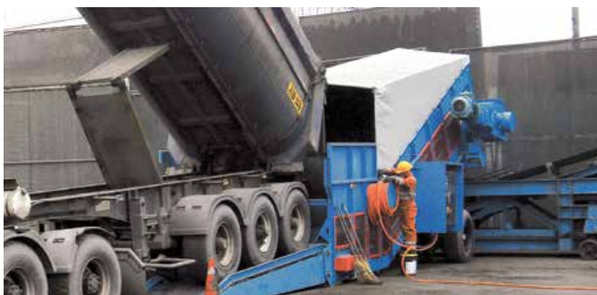
Independent Mobile Samson™ Material Feeder feeds an existing shiploader
