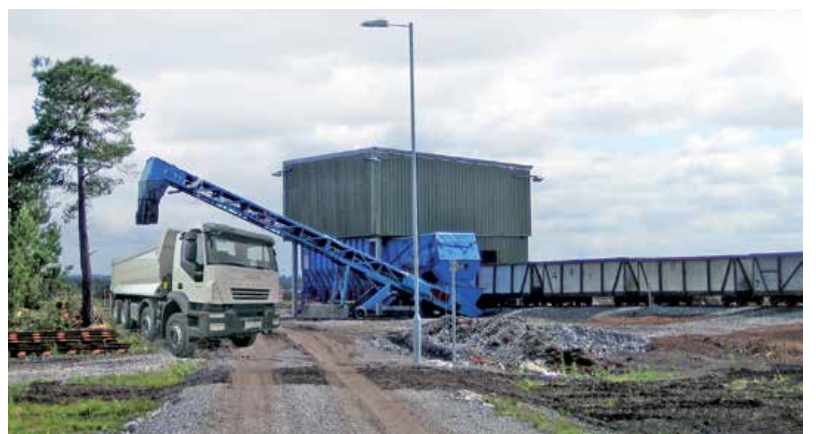
Transhipment from Rail Wagon to Tipping Truck
