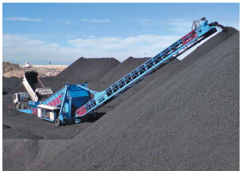
Stormajor™ Boom Feeder supplied with powered travel and hinged truck ramps for easy manoeuvring around the stackyard
