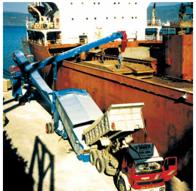
Shiploader + Stormajor™ Boom Feeder for truck to ship loading
