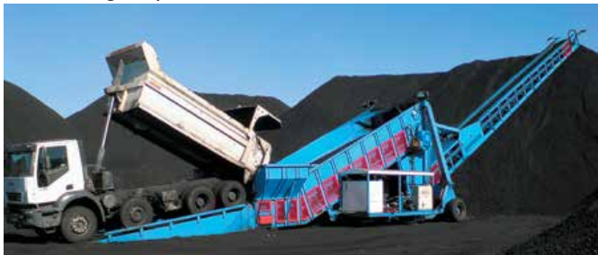
Mobile Stormajor™ Boom Feeder incorporates a Samson™ Material Feeder
