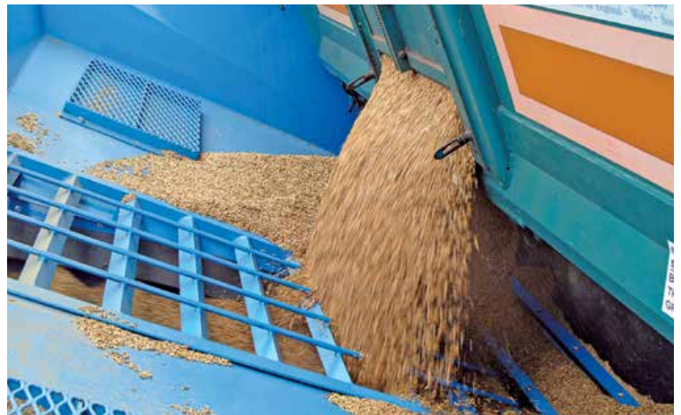
Regulated flow from the Truck Grain Door
