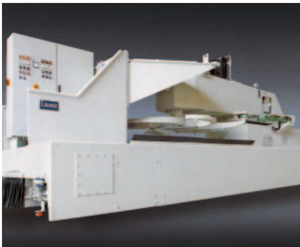
BEW with single side discharge and double swivel mechanism
