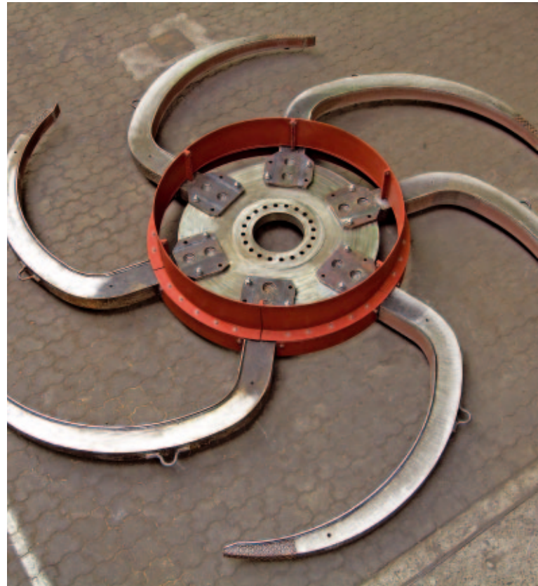
BEW-K discharge wheel, \varnothing 4,500 mm
