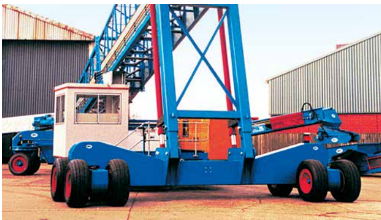
Forward axle beam with telescopic boom supports
