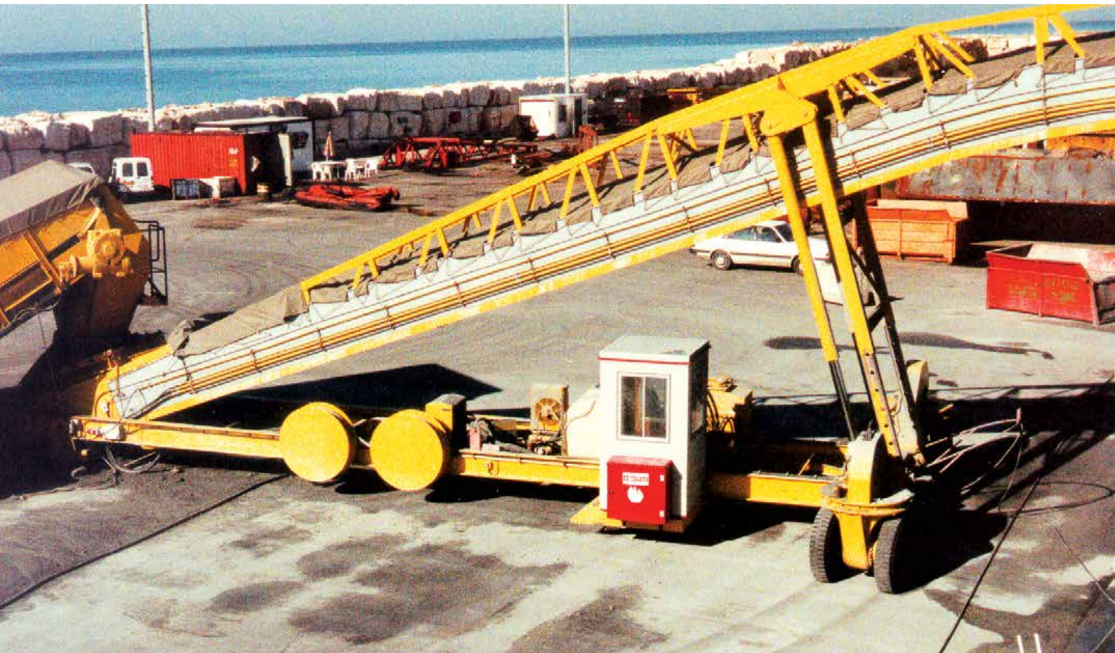
Powered radial operation with in-line tow travel
