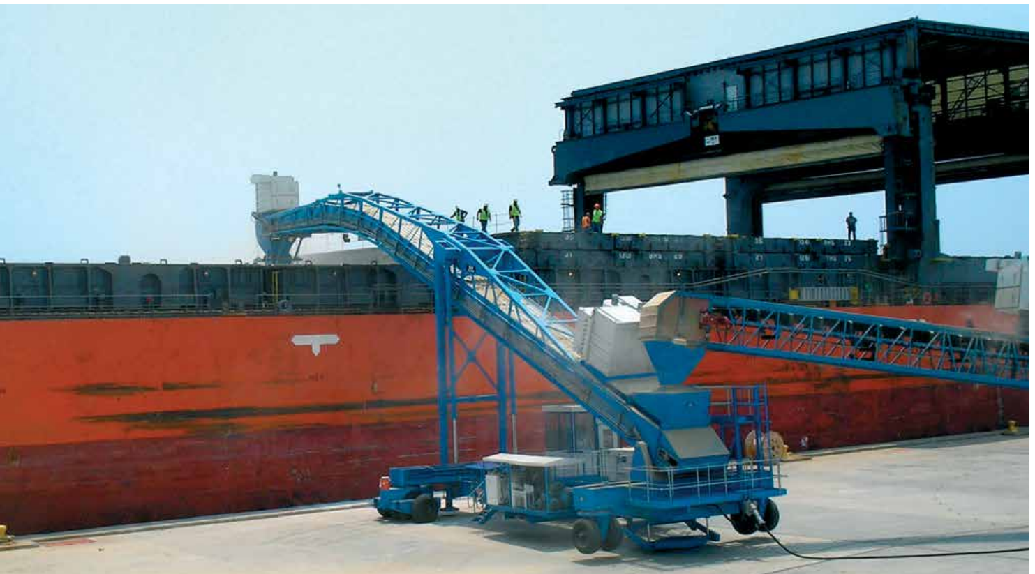
Shiploader with Radial Travel fed via Link Conveyor
