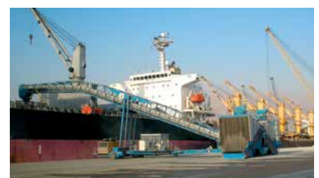
Shiploader with Twin Samson™ loading Panamax vessel
