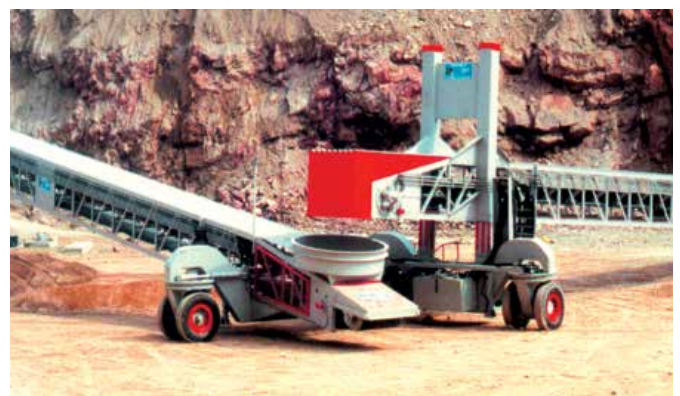
Link Conveyors with powered travel and full manoeuvring facilities
