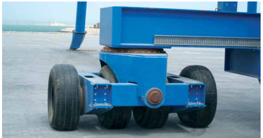
Four wheel pivoting axle assembly
