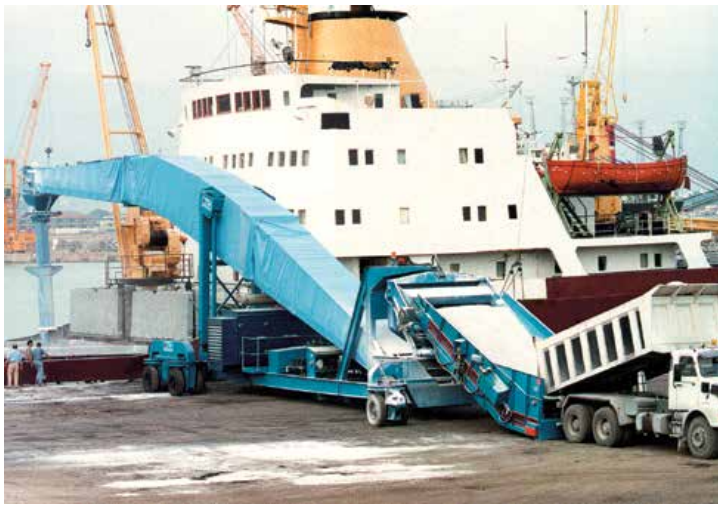
Slew Ring Mount allows the Samson™ Material Feeder to be positioned through 180 degree working arc
