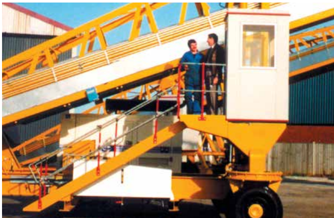
Operator's control cabin raised above the forward axle
