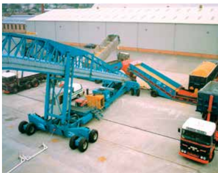
Twin independent Multi-Feed-Point Samson™ Material Feeders discharge to a single Shiploader
