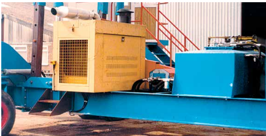
Auxiliary Gen-Set Drives the powered travel system only
