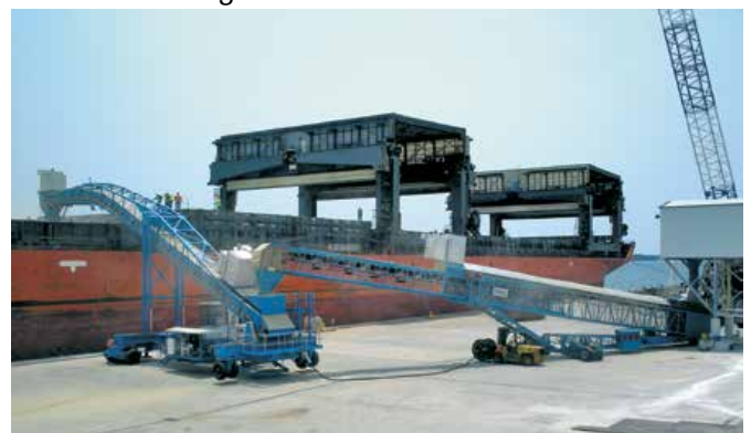
Shiploader with New Generation movement fed via Telescopic Link Conveyor
