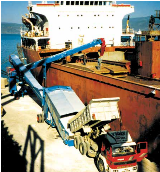
Raised chassis Shiploader with Stormajor™ Feeder
