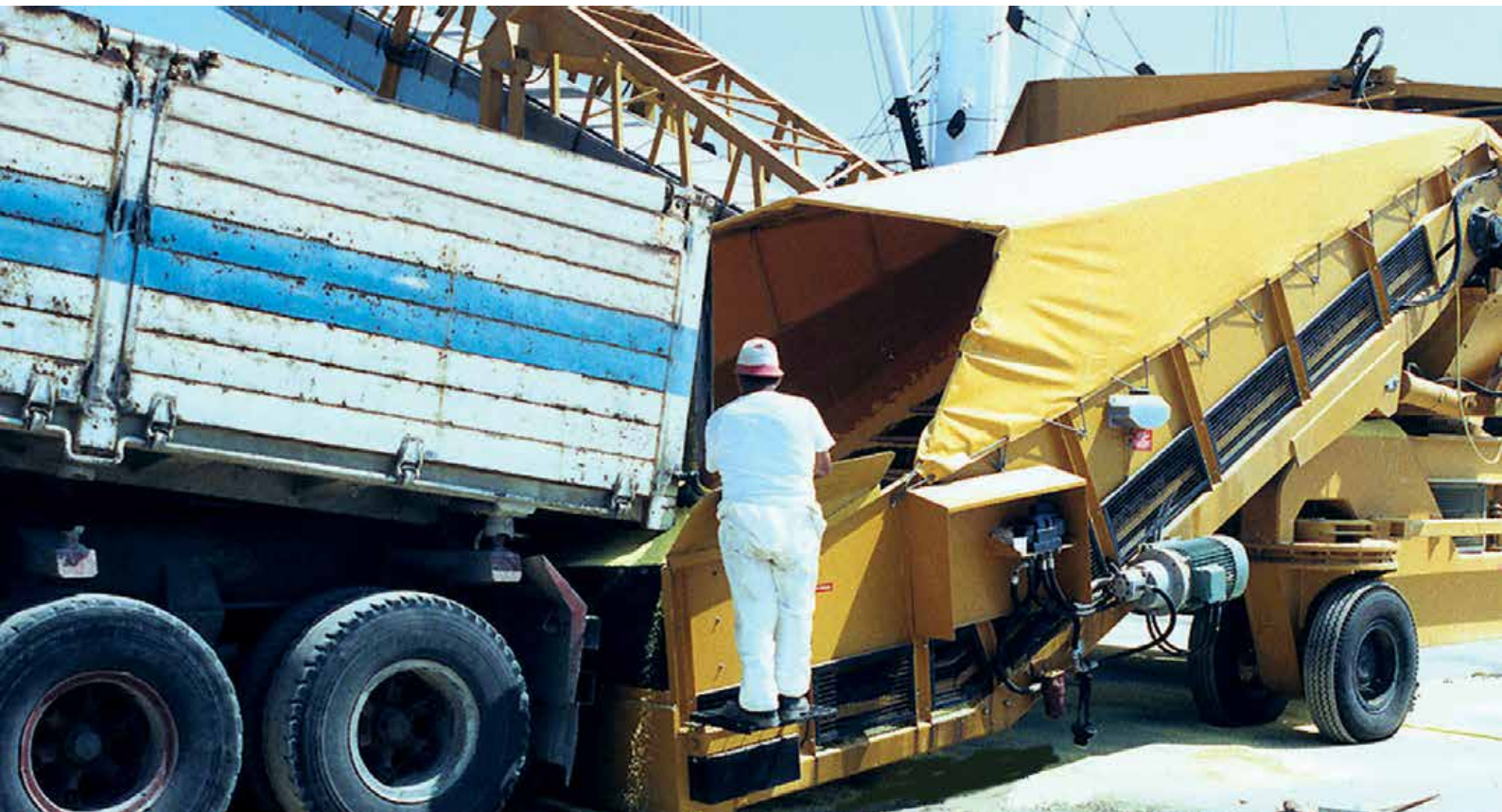
Tipping truck discharging direct to Mobile Samson™ Feeder – No Ramps Required
