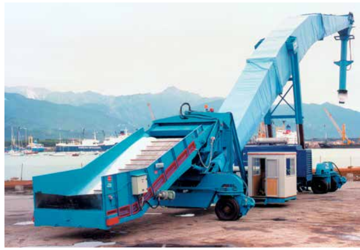
Samson™ Material Feeder raised for travelling
