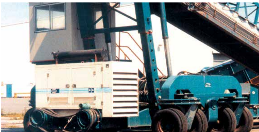
Combined Gen-Set and electric drive
