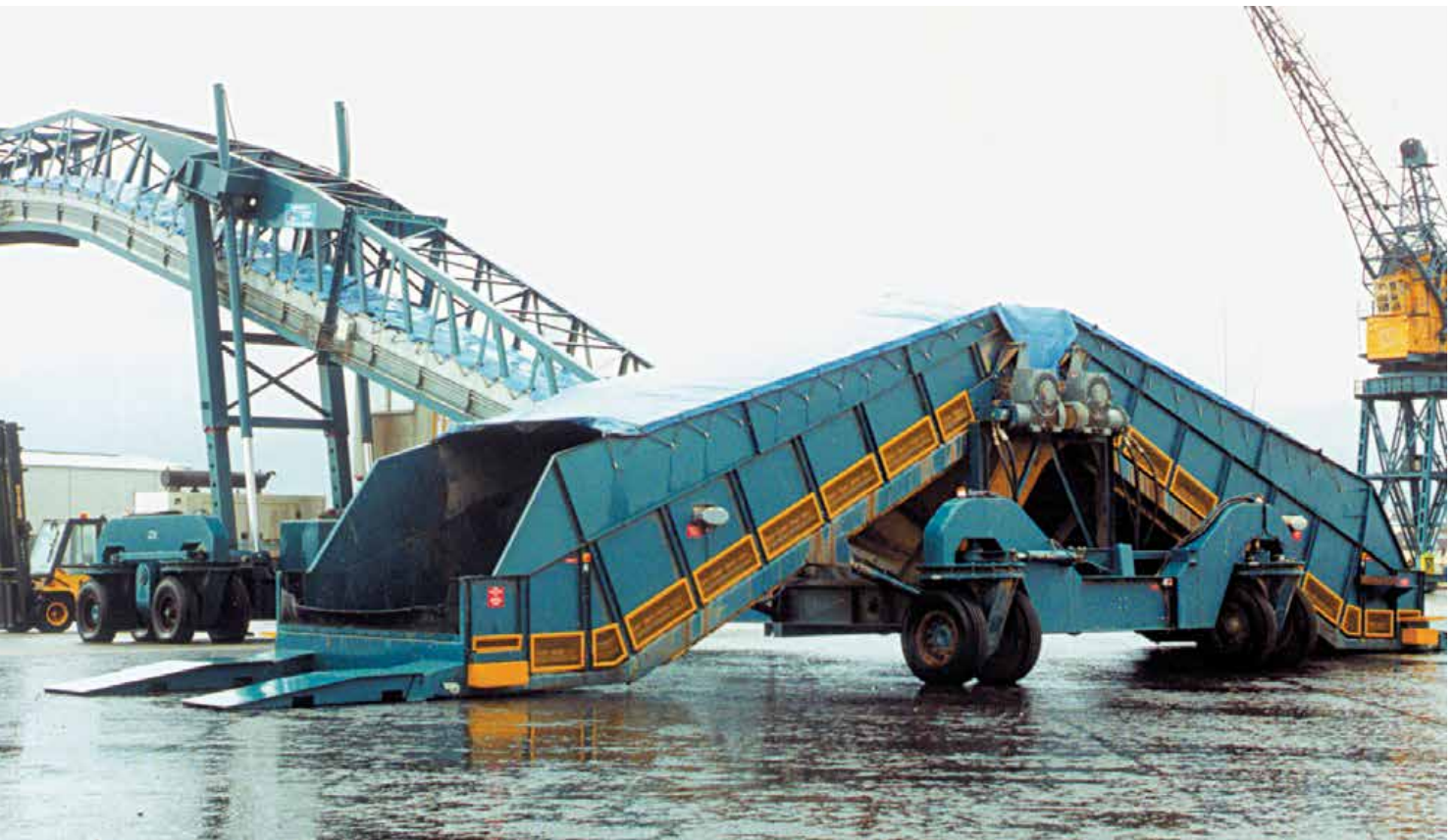
Twin Samson™ Material Feeders with flexible enclosures
