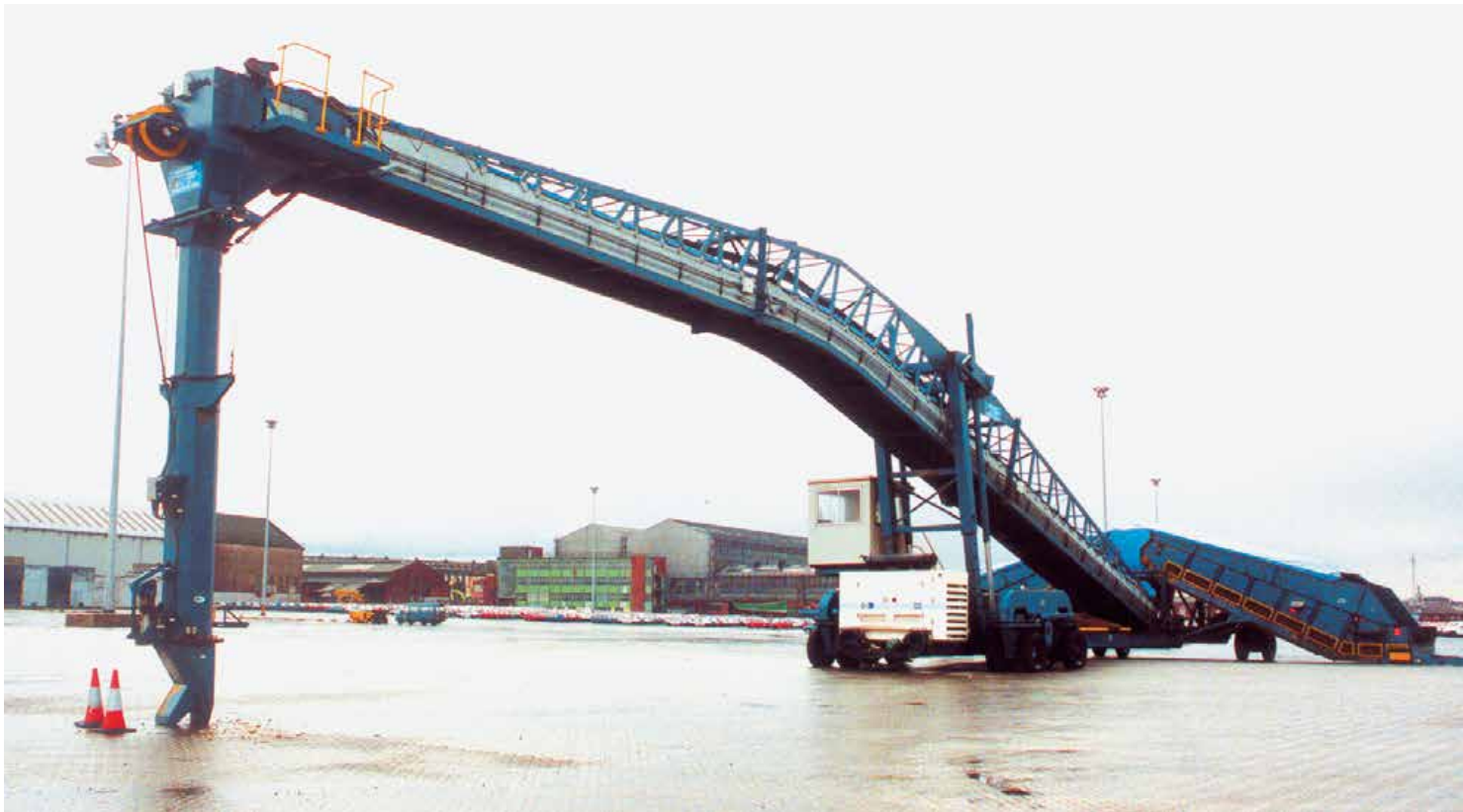
Full specification mobile Shiploader with a variable angle trimming chute and radial distributor
