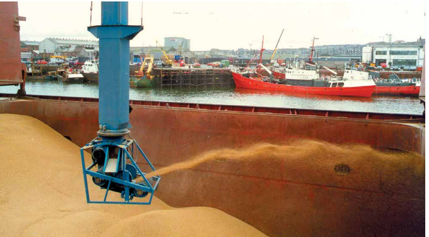
Radial thrower provides effective trimming with minimum machine movements
