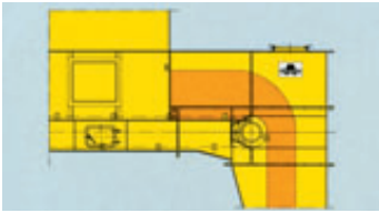
Overhead discharge for sticky materials
