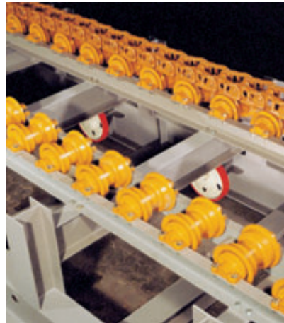
Fixed rollers for type BPB-S
