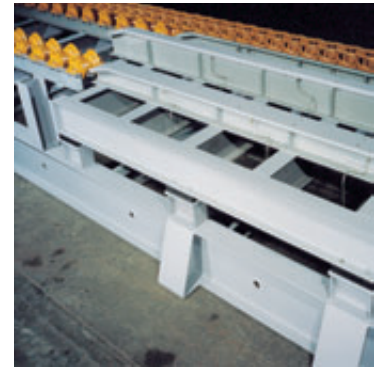
Impact table with shock absorbers
