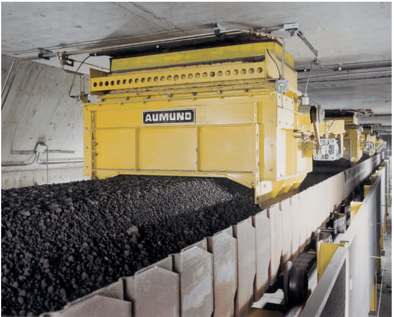
Silo Discharge with Remote Control
