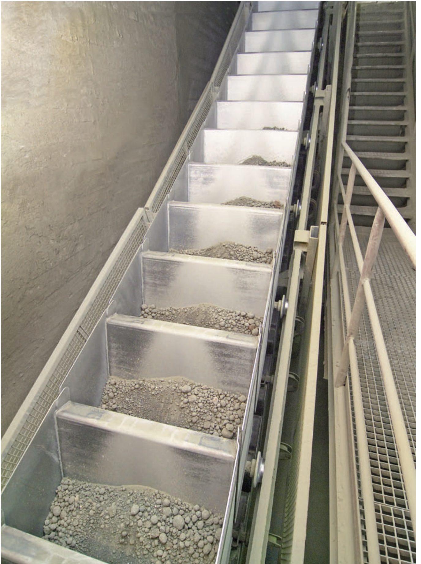
Clinker Transport with Conveyor type BZB
