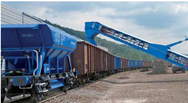
Mobile Stormajor™ loading to Rail Wagons
