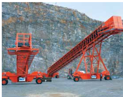
Two 50 metre x 1400 mm link conveyors
