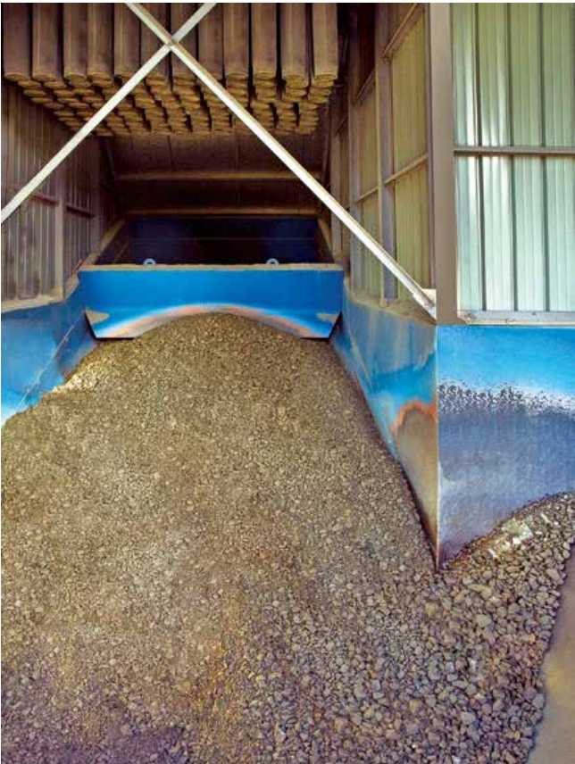
Minimum excavation but 120 tons live holding capacity
