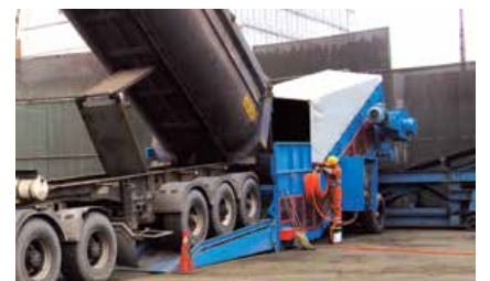
Independent Samson™ feeds an existing shiploader
