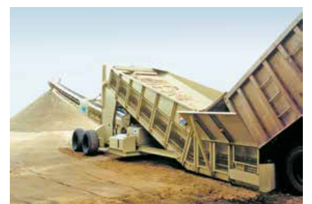
Direct receive from tipping or dump truck
