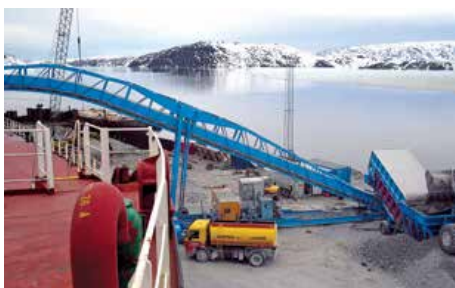
Cambered boom for maximum lift and outreach
