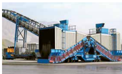
Simultaneous intake from two trucks
