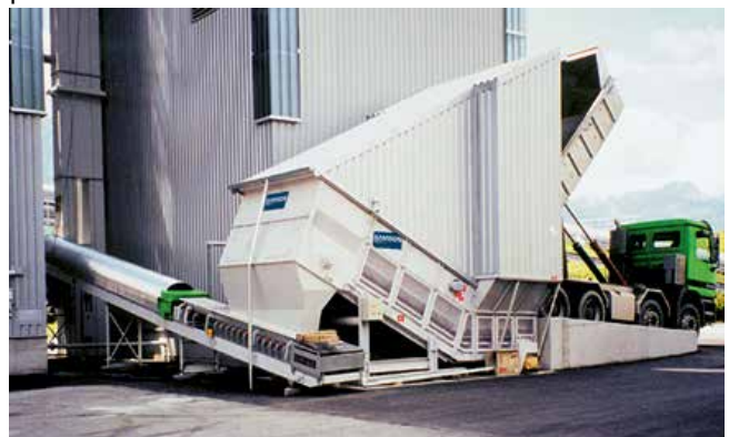
Surface installation eliminates deep pits underground hoppers and offering maximum flexibility in location
