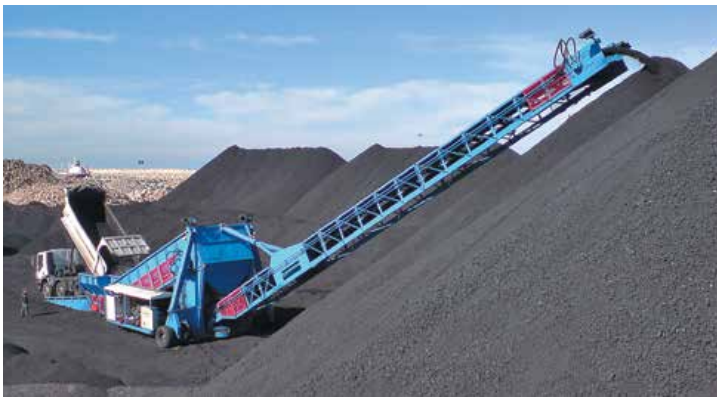
Mobile Stormajor™ direct from tipping truck to stockpile
