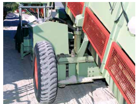
Powered travel and steering for easy travel along the rake
