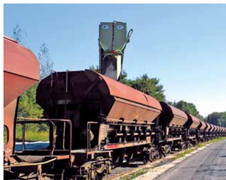
Rotating loading chute for accurate material placement
