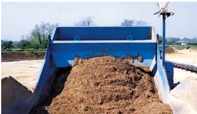
Levelling blade output control for regulated feed rate
