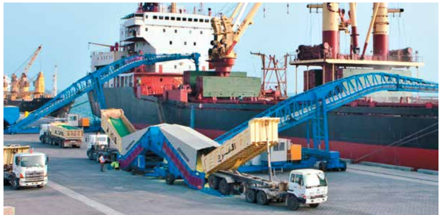
Twin Independent Samson™ units feed a single Shiploader
