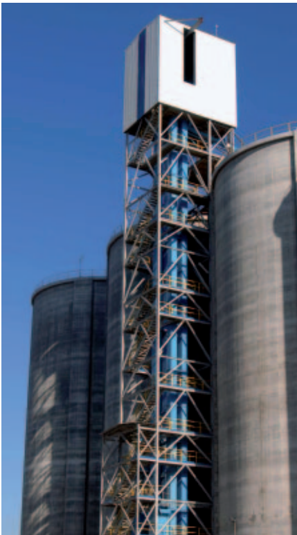
Belt Bucket Elevators for material size to 10 mm and temperatures to 130°C
