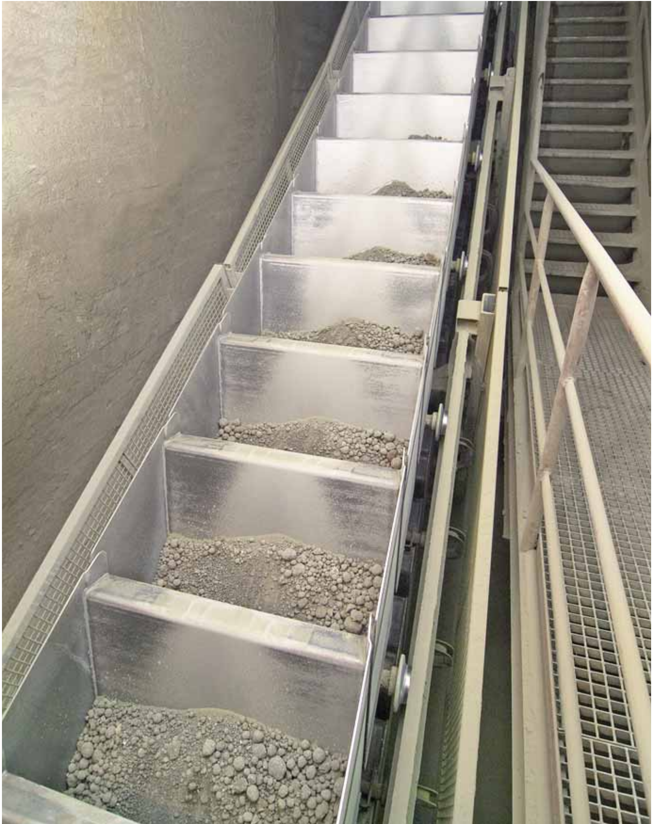
Clinker Transport with Conveyor type BZB
