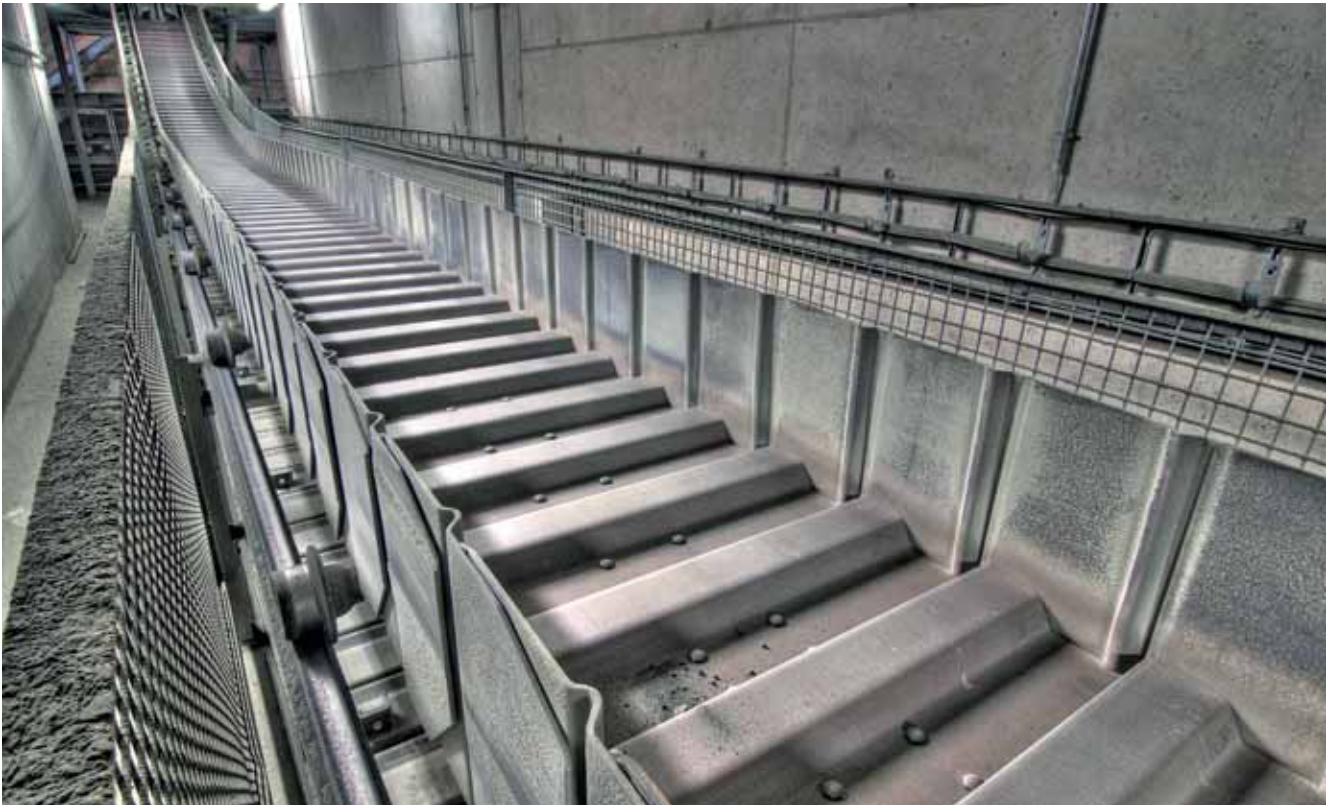
Pan Conveyor type KZB - Detail
