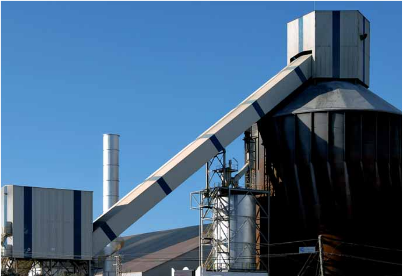
Pan Conveyor KZB-Q connecting cooler and silo
