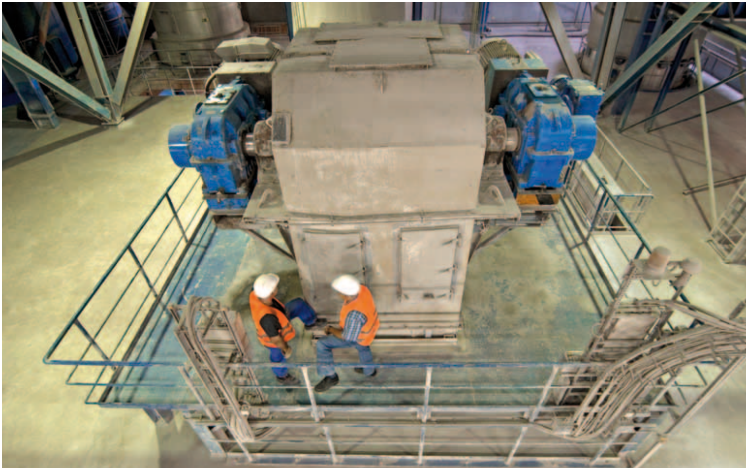
Head of Double Bucket Elevator with double drive and two bucket strands
