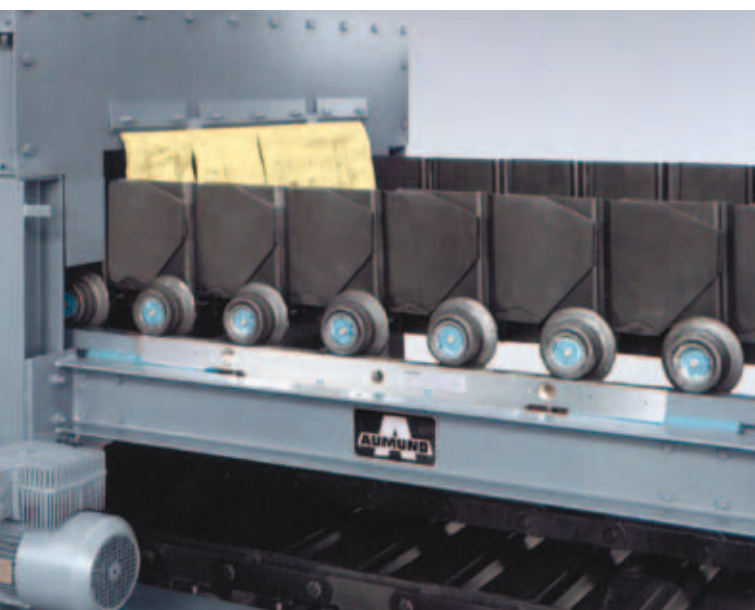
Apron Weigh Feeder with deep drawn pans
