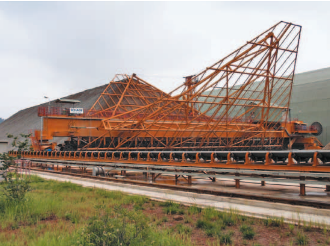
Bridge Scraper Reclaimer for limestone
