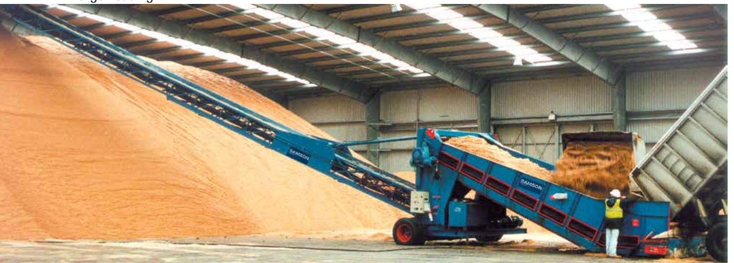
Stormajor™ combines the benefits of a Samson™ Material Feeder with a Radial Stacking Boom mounted to a common mobile chassis
