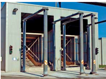
Twin Samsons™ Material Feeder with Traffic Management
