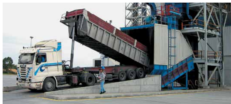
Samson™ Material Feeder Clinker Intake for Cement Grinding Plant with integrated Dust Extraction
