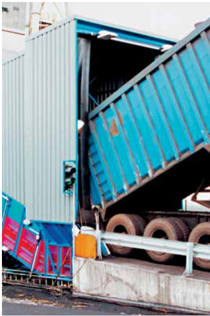
Wide belt design eliminates bridging
