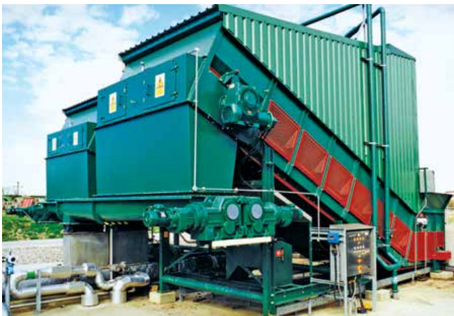
Twin Screws meter output to progressive cavity pump
