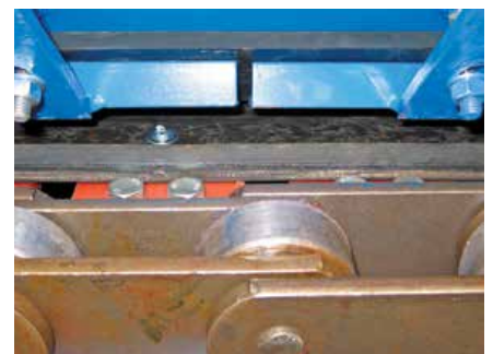
Load carried on the chain rollers
