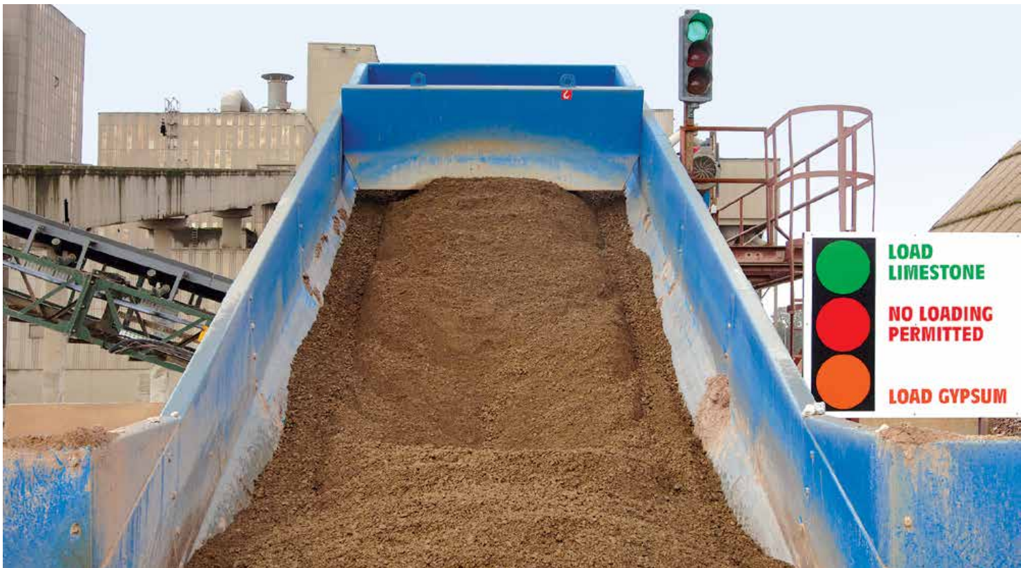
Material stored within the Samson™ Material Feeder body may be at various load levels along the length of the unit
