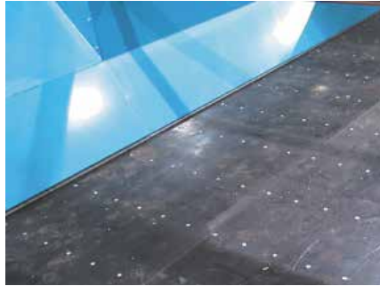
Wide belt design eliminates bridging
