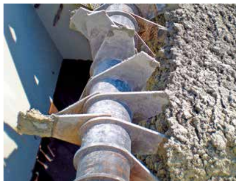
Rotating teaser provides a closely controlled discharge rate handling wet clay
