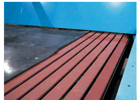
Steel Apron Bars support the load
