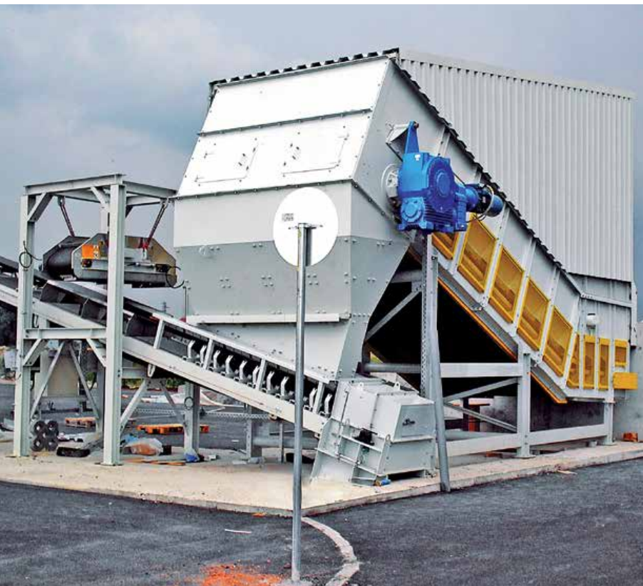
Samson™ Material Feeder with teaser discharges to an Inclined belt conveyor
