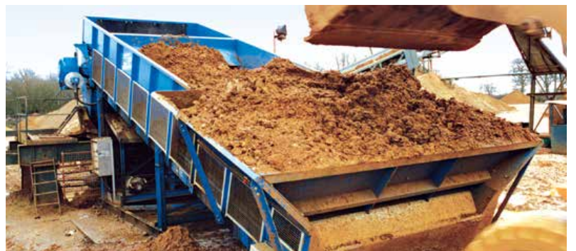
The Samson™ Material Feeder with Straight Chassis and Flared Entry (width 4.5 m) receives sandy clay from shovels
