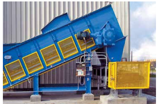
Synthetic Gypsum discharged to horizontal belt conveyor
