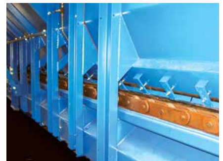
External chains outside the material flow
