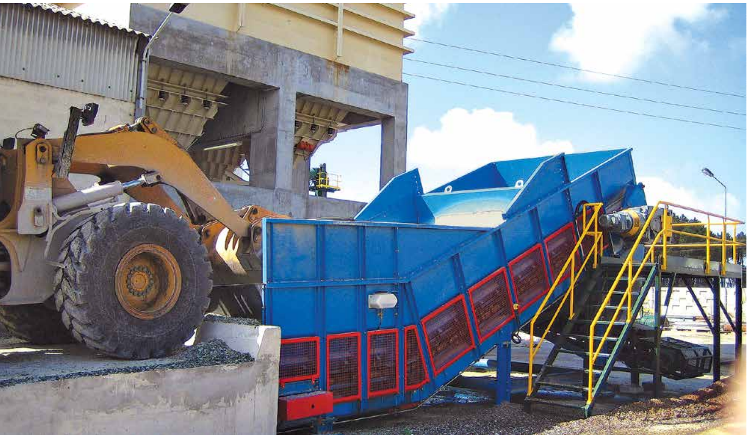
The Samson™ Material Feeder with deflected chassis and parallel entry (width 3.0 m) receives broken glass from both tipping trucks and shovels
