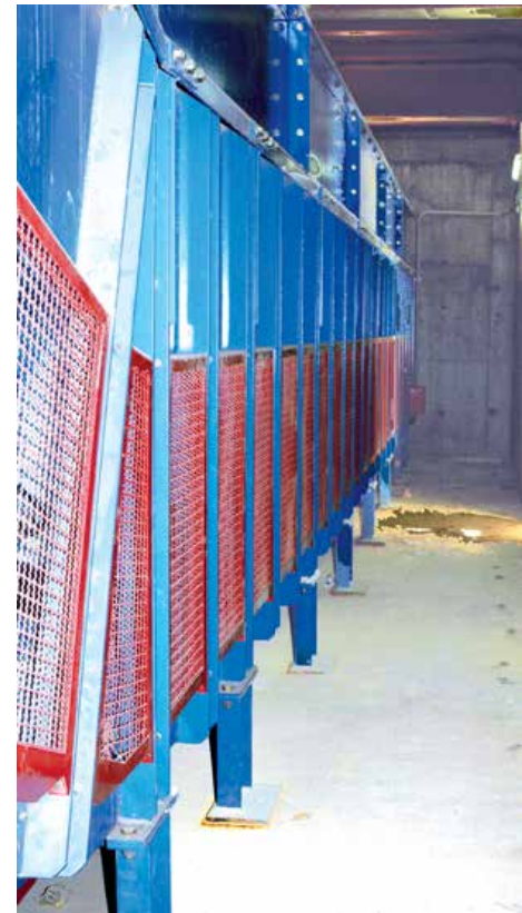
Discharge facility for Hopper Bottom Railcars receives coal for a Cement Plant including a Samson™ Material Feeder with 80 tons holding capacity
