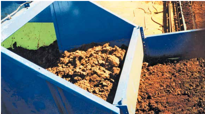
Levelling blade controls the material bed depth at the discharge
