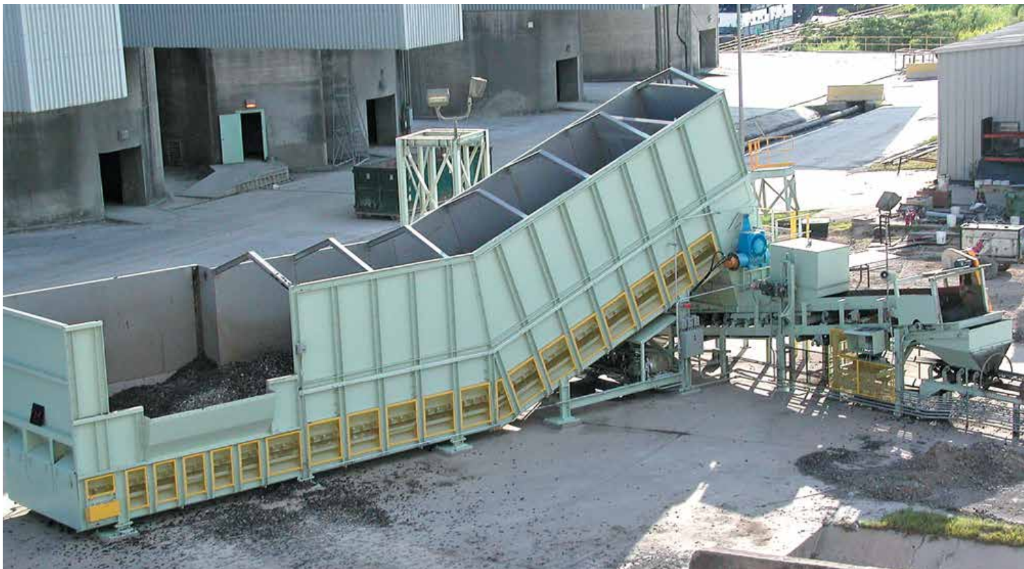
The Samson™ Material Feeder MF08xxx Series provides 100 cubic metres of live storage for Alternative Fuels in a Cement Plant
