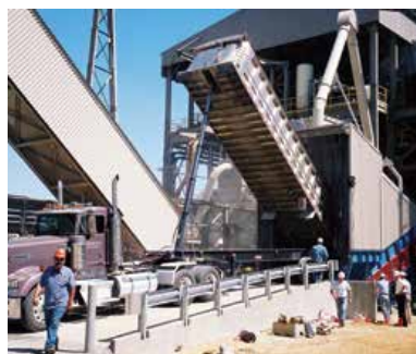
Full enclosure with ducted dust extraction
