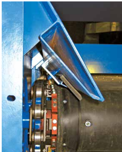
Flexible side seal with outer belt ledge
