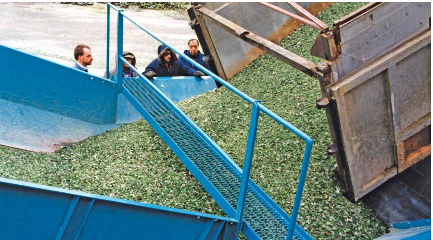
Broken Glass is received by the Samson™ Material Feeder at a Recycling Operation
