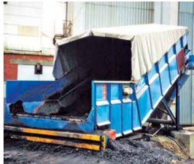
Flexible PVC sheet partial enclosure
