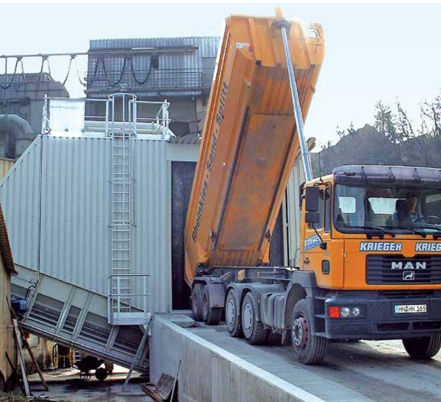
The Side Loading Samson™ Material Feeder receives Cement Clinker for import directly to an existing conveyor installation
