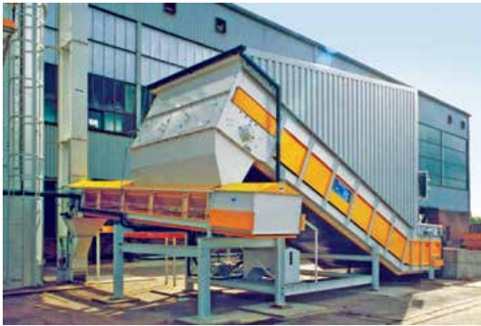
Kleen-Line Belt Feeder transfer to Bucket Elevator
