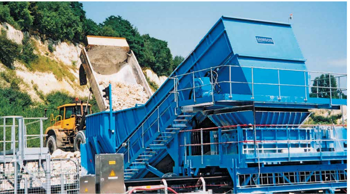
Samson™ Material Feeder plus Twin Shaft Rotary Sizer receives as-mined Limestone from dump trucks and provides a manageable lump size for onward conveying
