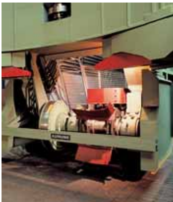
Internal Ring with Thrust Bearings and Travel Unit
