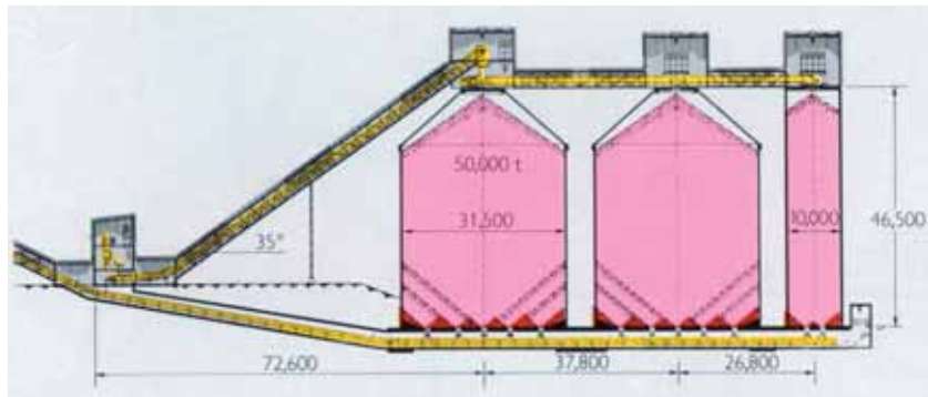
Clinker Silos in Series
