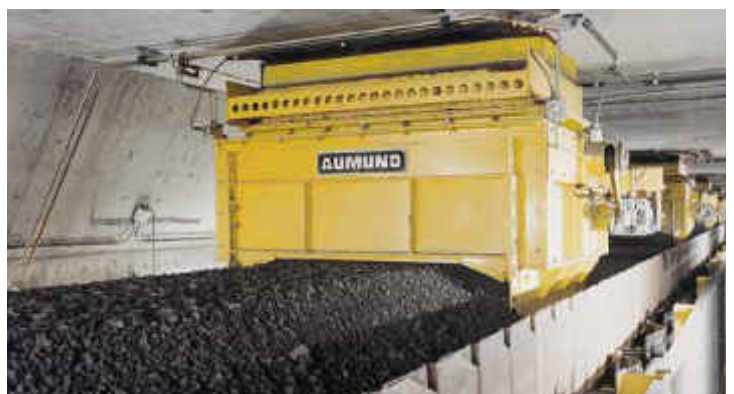
Gravity silo discharge
