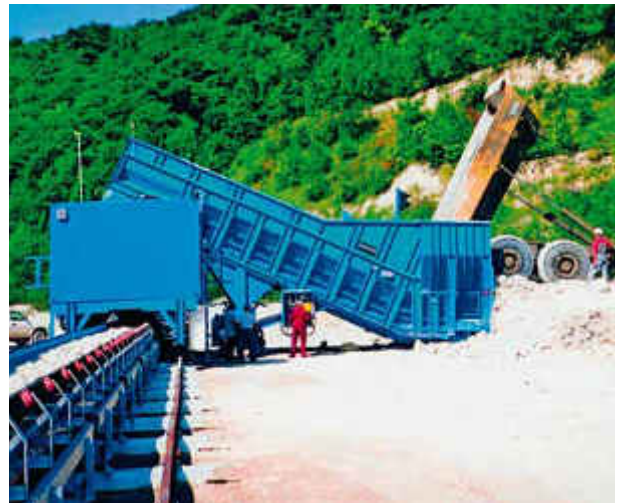
Samson® Feeder - for crusher feeding in a quarry
