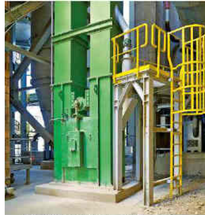
Elevator boot with parallel tensioning device
