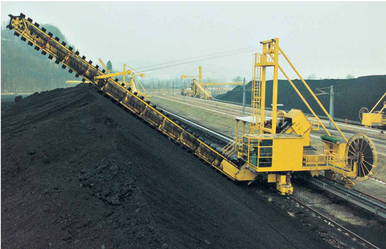
Cantilever Scraper Reclaimer designed for frozen Coal
