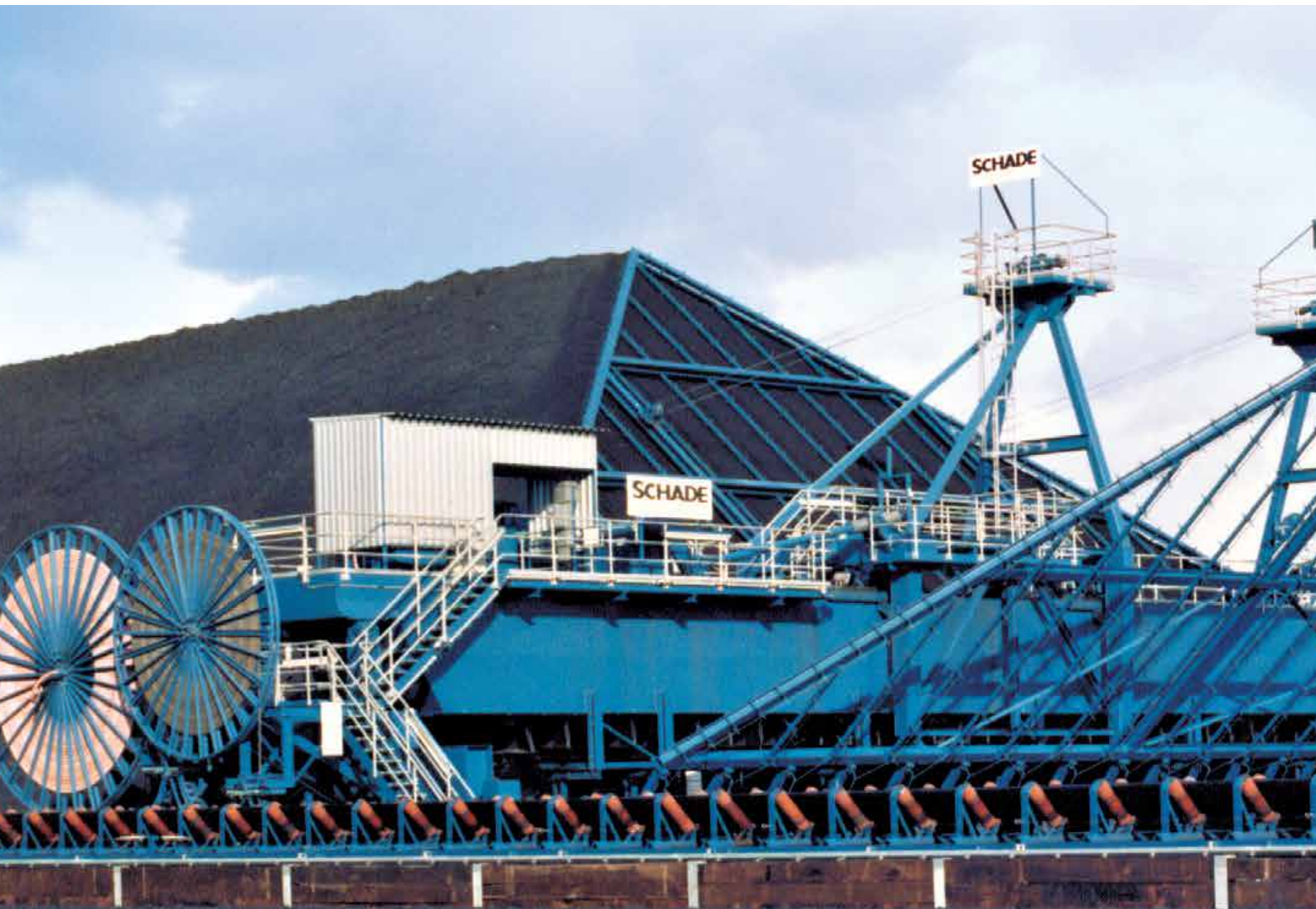
Bridge Scraper Reclaimer, 50 m span, 1,100 t/h, Coal
