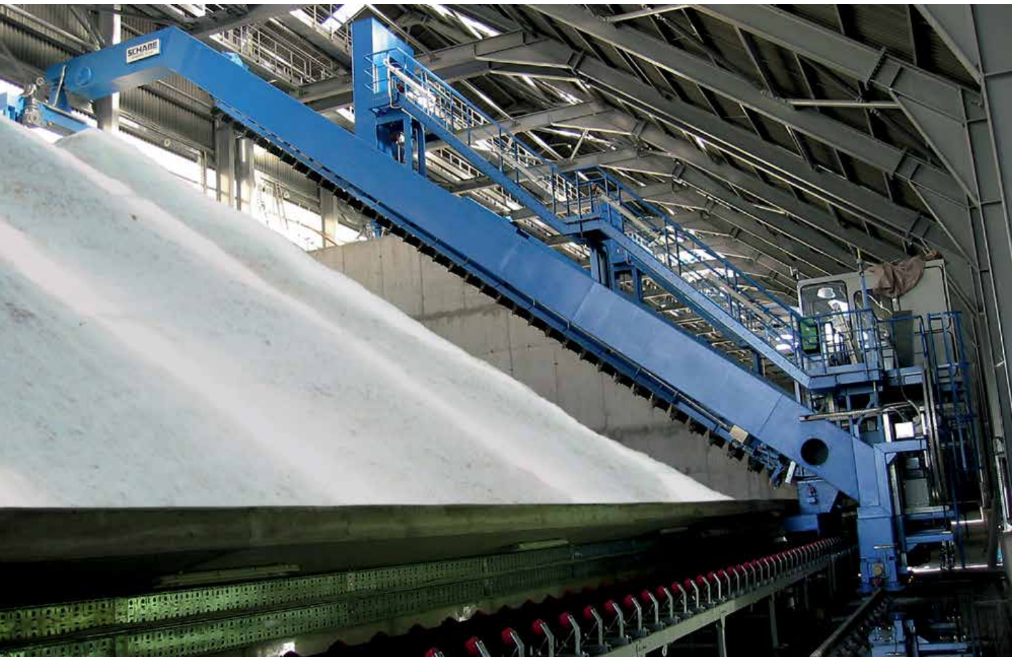
Portal Scraper Reclaimer, 21 m span, 150 t/h, additives
