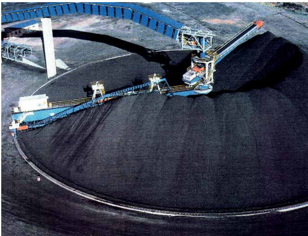
Circular Stacker / Bridge Scraper Reclaimer, rail dia 104 m, stacking 1,200 t/h, reclaiming 1,200 t/h, Coal
