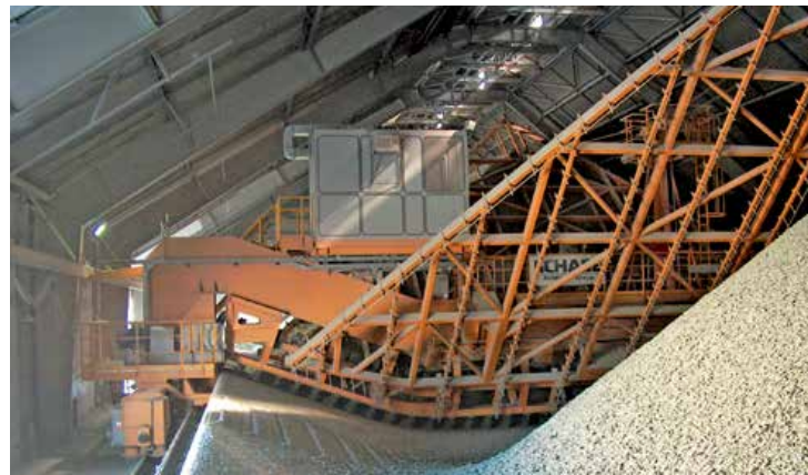
Bridge Scraper Reclaimer, 27.5 m span, 300 t/h, Gypsum
