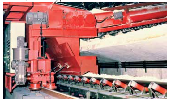
Direct discharge on belt conveyor
