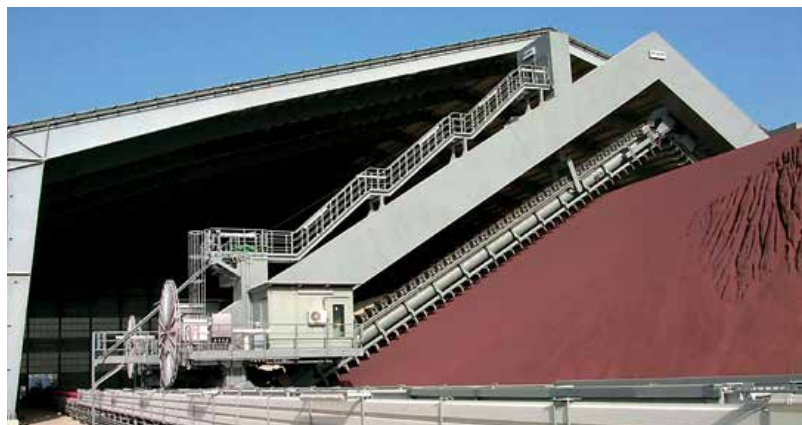
Portal Scraper Reclaimer, 49 m span, 550 t/h, additives
