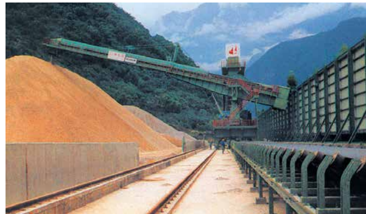
Fig. 3 Luffing Stacker for 2,000 t/h Limestone
