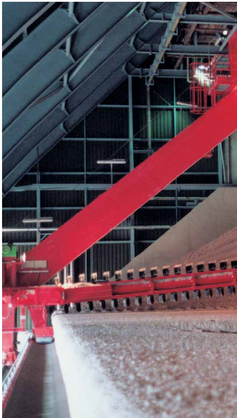
Portal Scraper Reclaimer, 32 m span, 400 t/h, FGD-Gypsum
