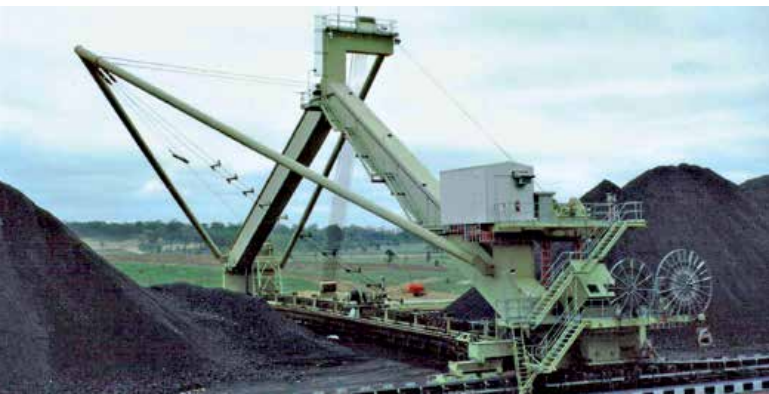
Portal Bridge Reclaimer, 50 m span, 600 t/h, Coal
