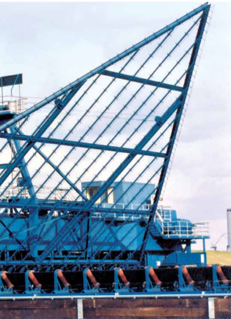
Bridge Scraper Reclaimer, 26.4 m span, 250 t/h, Limestone
