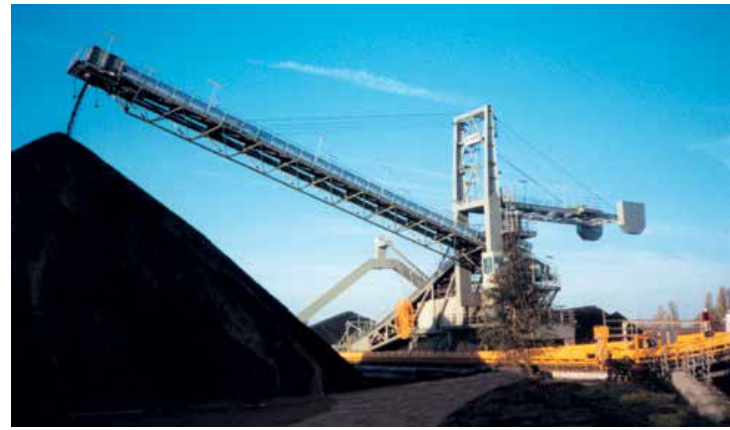
Fig. 2 Slewing/Luffing/Stacker for 1,000 t/h Coal
