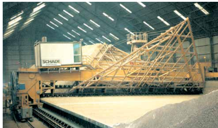
Bridge Scraper Reclaimer, 26.4 m span, 250 t/h, Limestone
