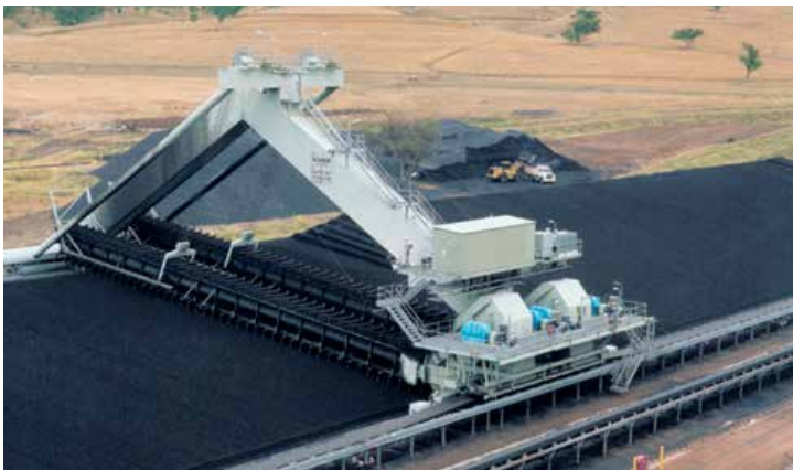
Portal Scraper Reclaimer with twin booms, 52 m span, 3,100 t/h, Coal
