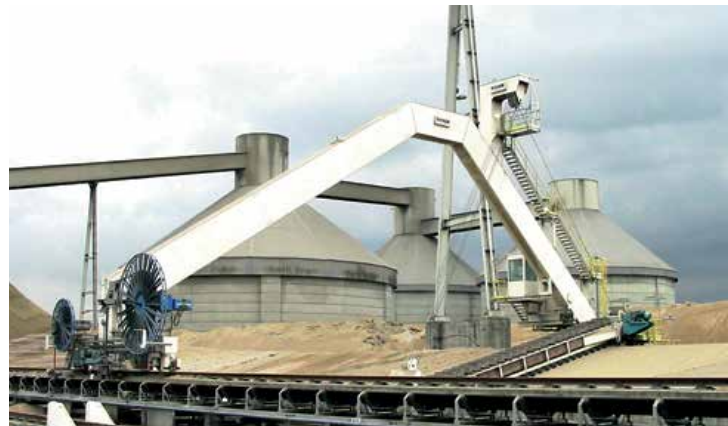
Portal Scraper Reclaimer, 33 m span, 600 t/h, slag
