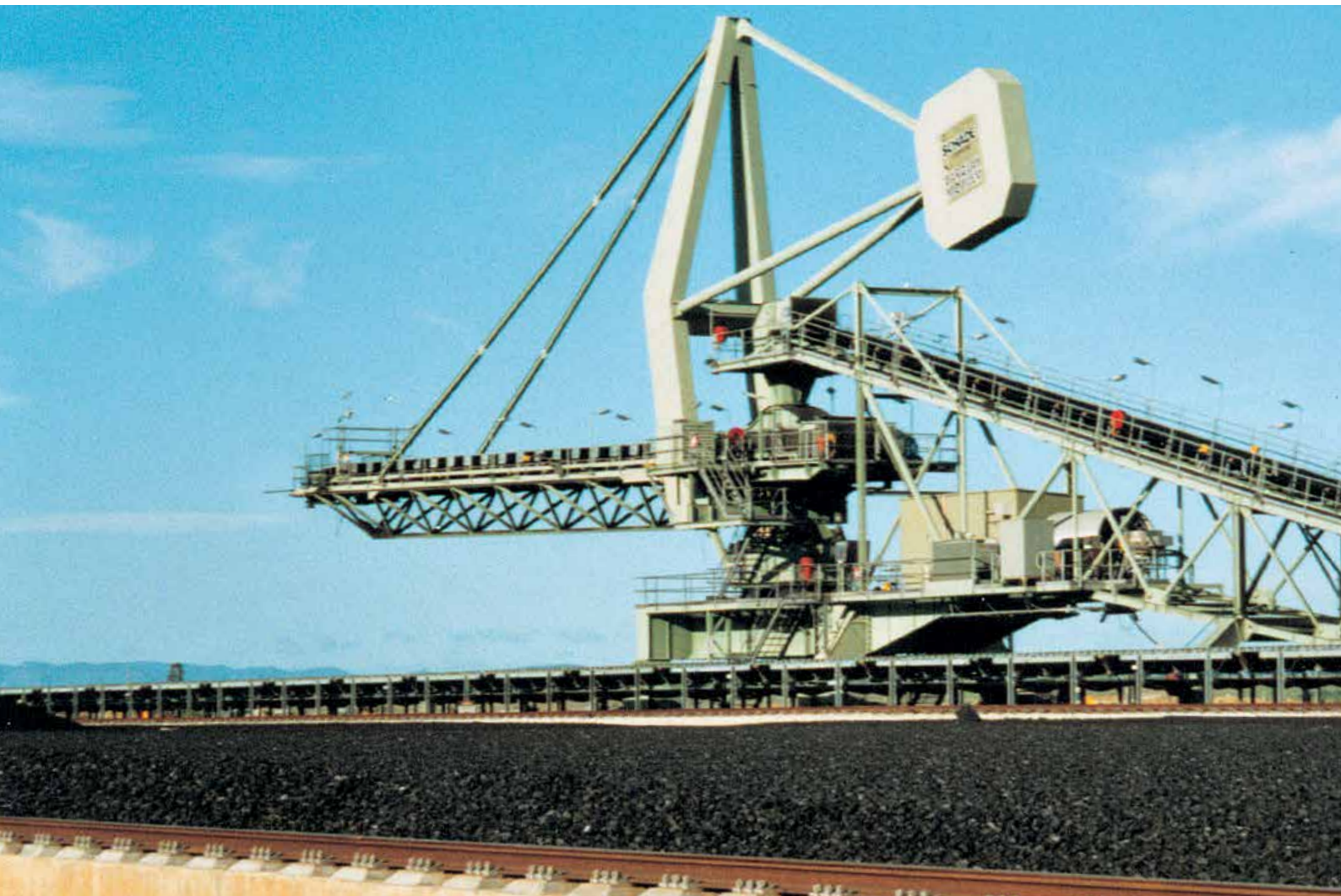
Fig. 1 Slewing/Luffing/Stacker for 2,750 t/h Coal
