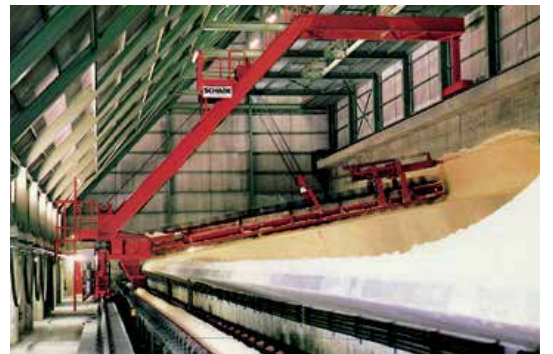
Semi Portal Scraper Reclaimer, 14 m span, 80 t/h, FGD-Gypsum
