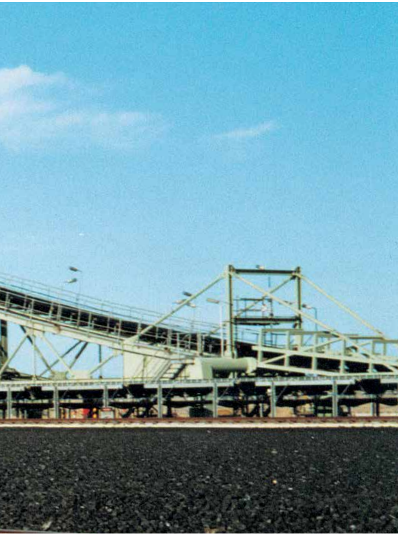
Fig. 2 Slewing/Luffing/Stacker for 1,000 t/h Coal
