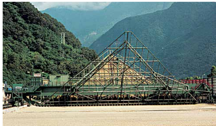
Bridge Scraper Reclaimer, 56 m span, 1.200 t/h, Limestone
