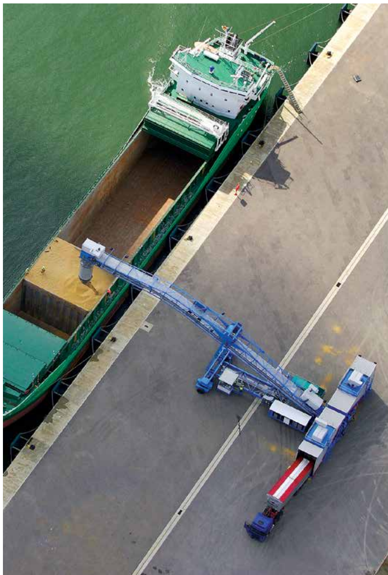
High performance Mobile Shiploader operates on any berth and may be moved clear for other port operations
