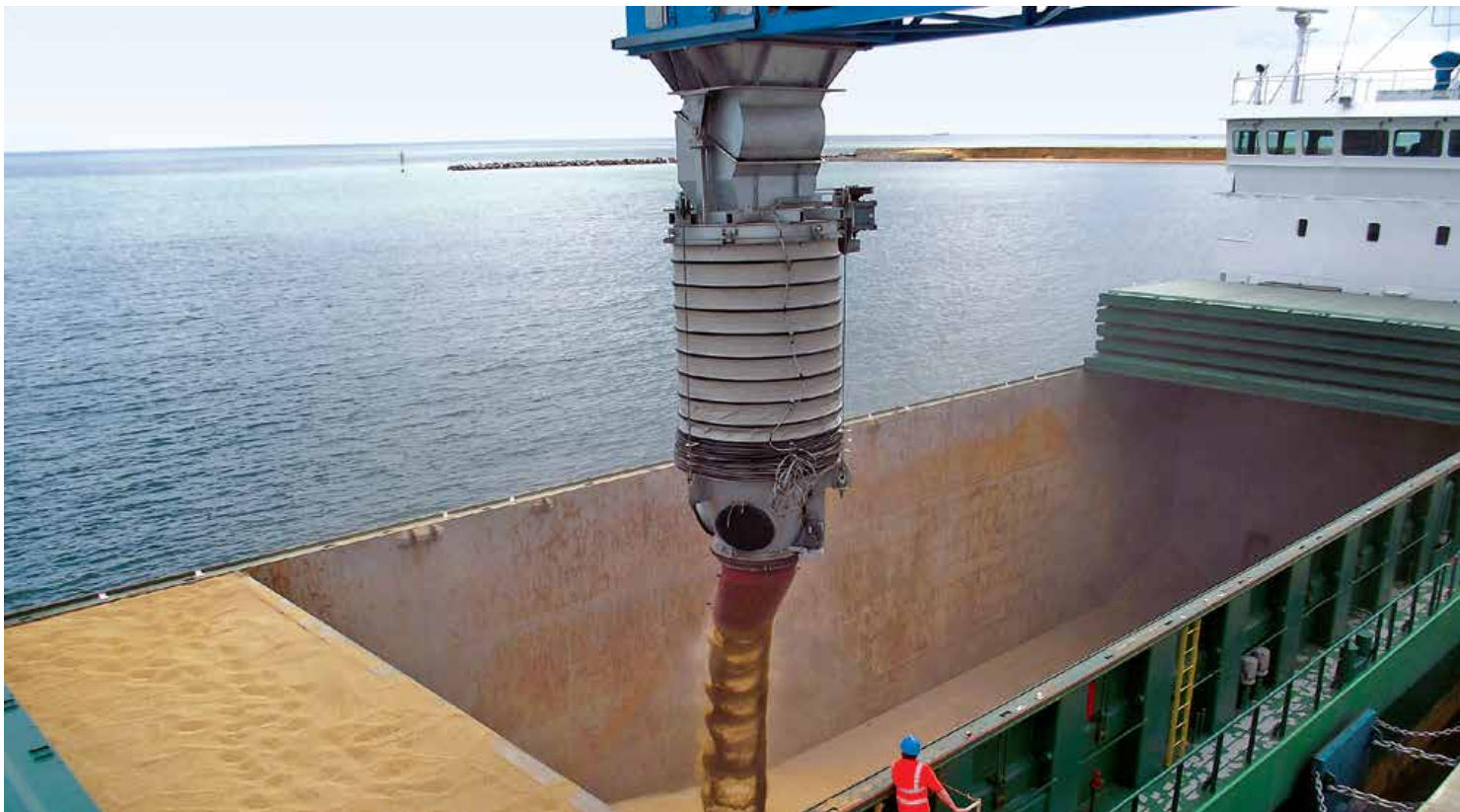
Rotating Trilling Chute for accurate material placement
