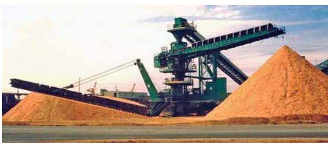
Circular Storage with Cantilever Reclaimer by SCHADE
