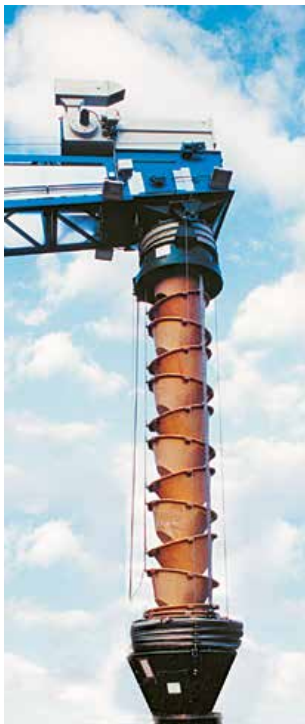
Telescopic Cascade Trimming Chute comprising a stack of inclined cones control the material flow velocity therefore prevent particulate separation controlling dust generation at the source
