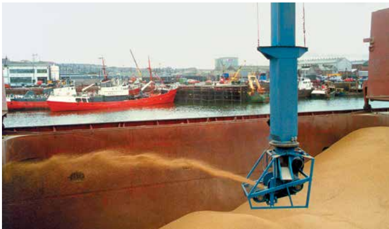
Where dust is not an issue, the Radial Jet-Slinger is an effective Ship Trimmer
