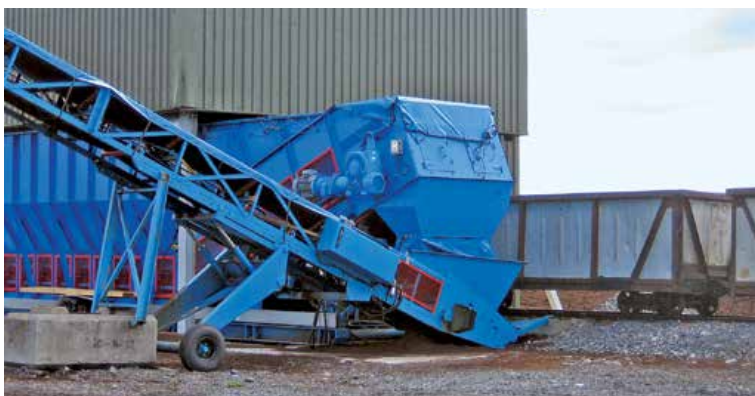
Discharge Direct from Samson™ Box Feeder to Mobile Conveyor
