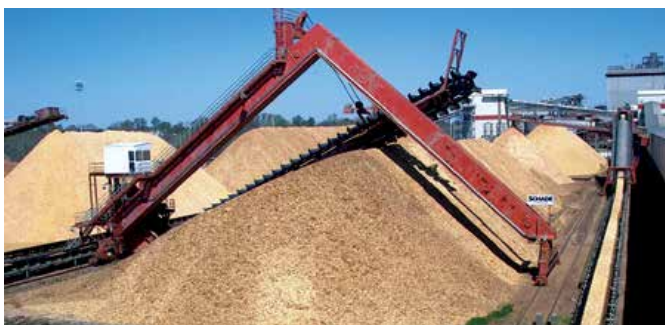
Longitudinal Storage with Portal Reclaimer by SCHADE
