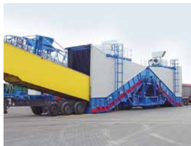
Twin Samson™ Material Feeders mounted to the Shiploader
