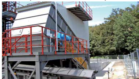
Weigh Belt Feeder gives Close Output Control
