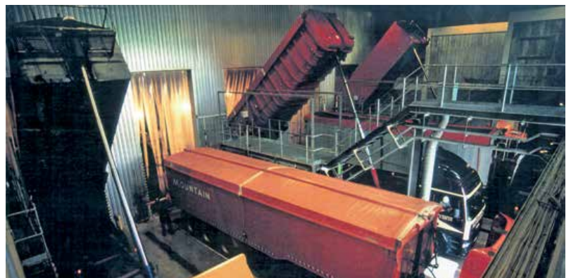
Samson™ Receiving Unit with Levelling Blade output control Disk Screen and Sub-Screen Feeder
