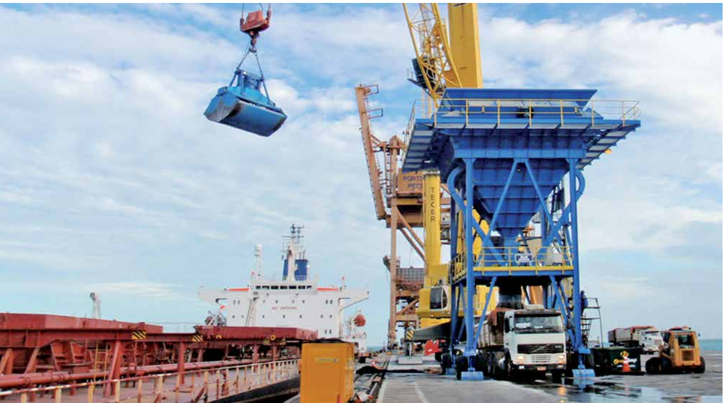
Eco Hopper discharges direct to trucks for movement to inland storage
