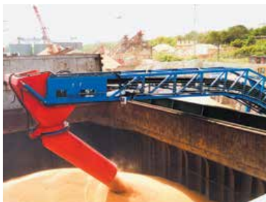
Twin Samson™ Material Feeders mounted to the Shiploader
