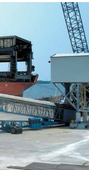
Twin SAMSON™ Feeders Discharging to a Mobile Ship Loader
