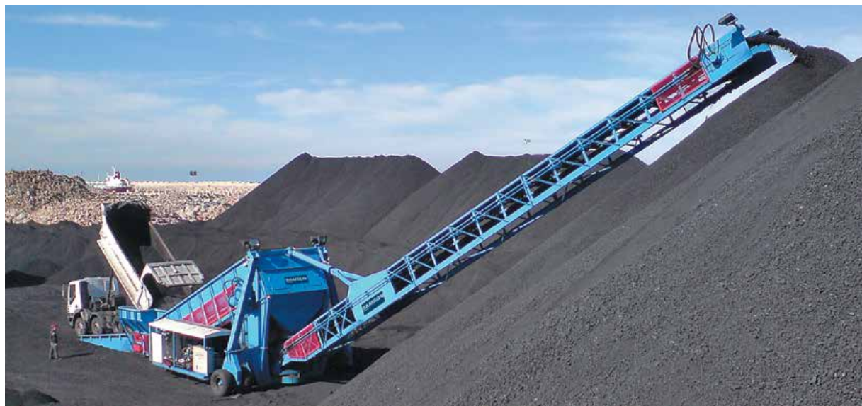
Stormajor™ Radial Boom Stacker with integral SAMSON™ Surface Feeder at an open Stockpile
