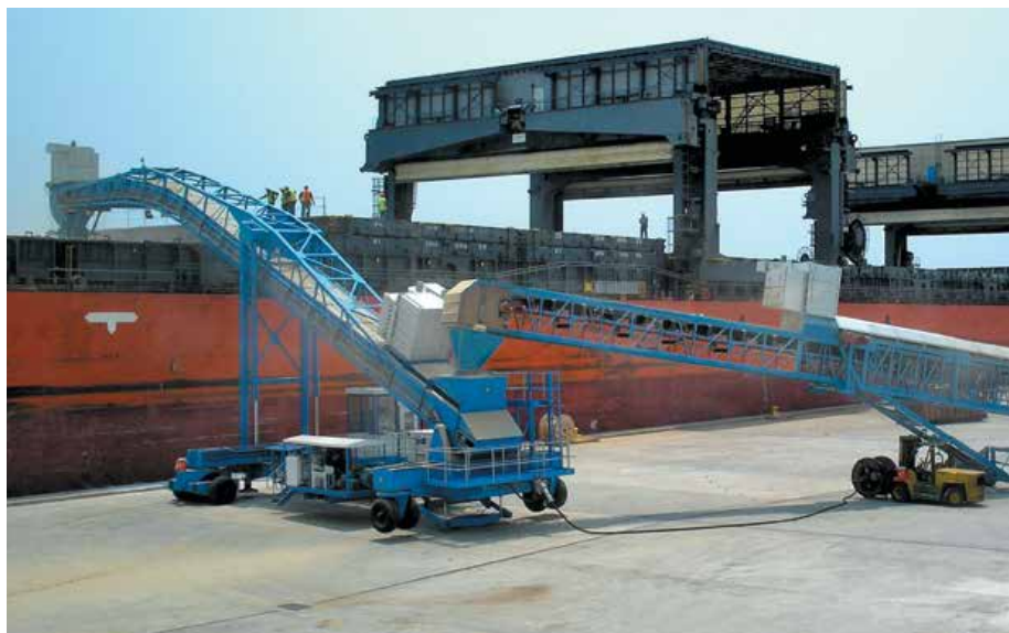
Mobile Shiploader with Mobile Telescopic Link Conveyor
