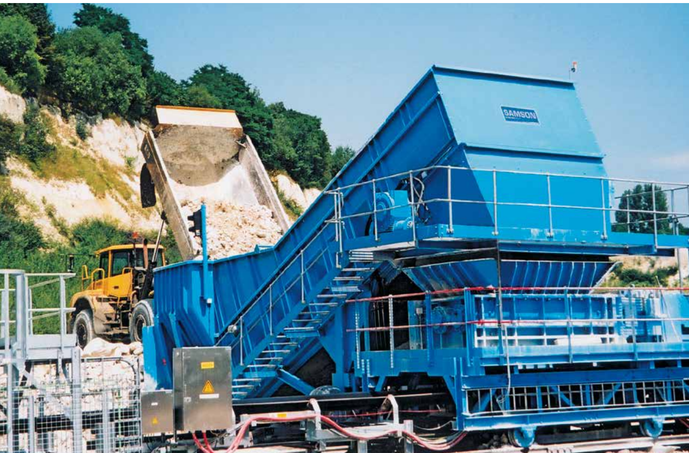
SAMSON™ Surface Feeder with Integrated Crusher
