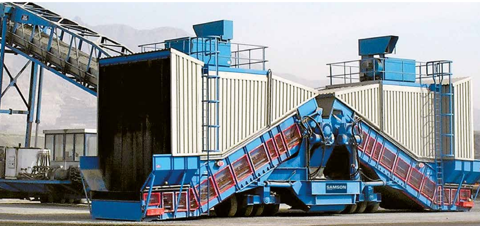
Twin SAMSON™ Feeders Discharging to a Mobile Ship Loader
