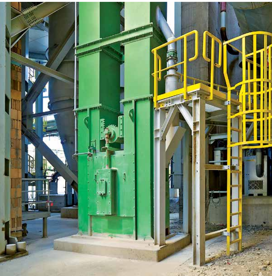
Elevator boot with parallel tensioning device
