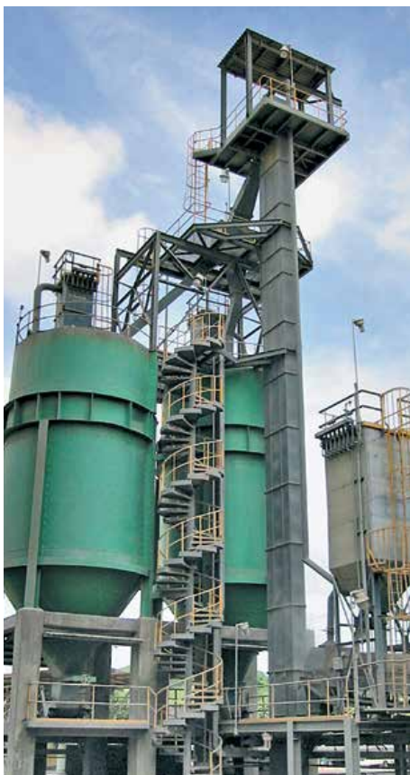
Bucket Elevator Type BWZ handling pozzolana and limestone
