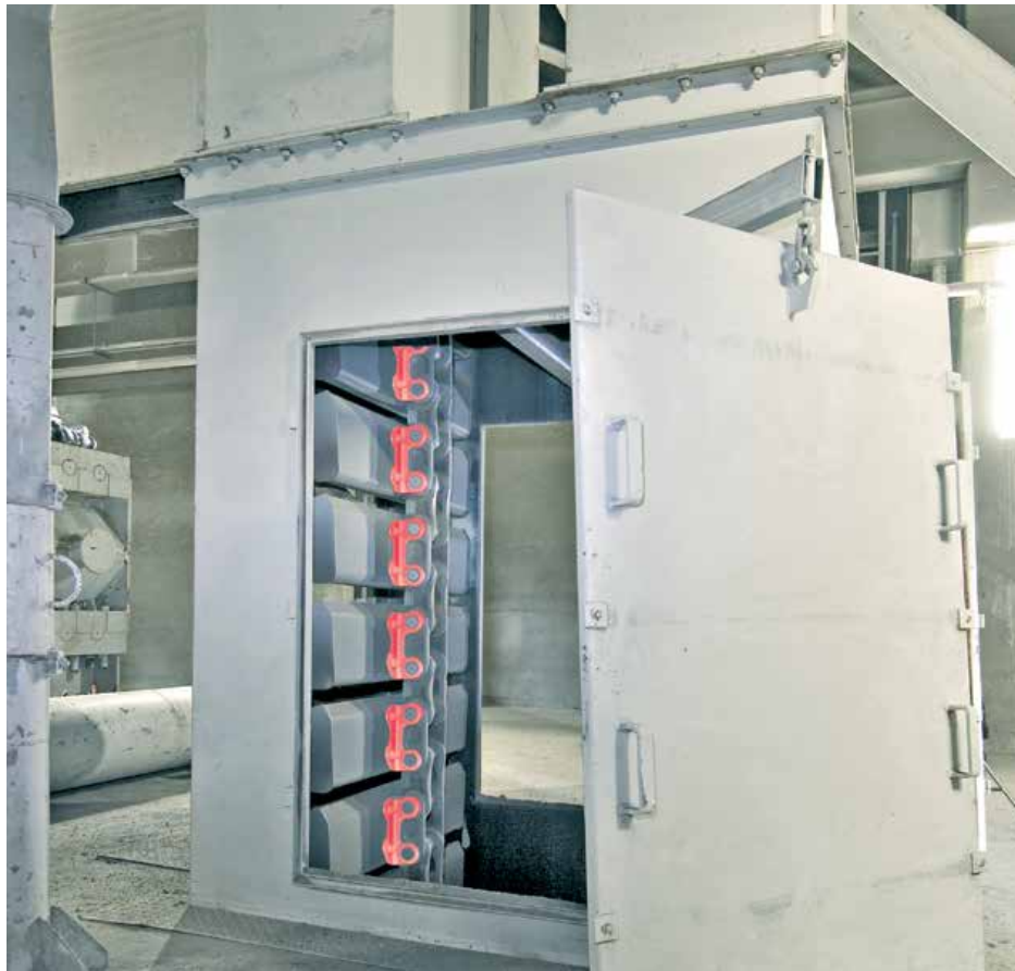
Assembly casing with hinge-supported door for easy maintenance
