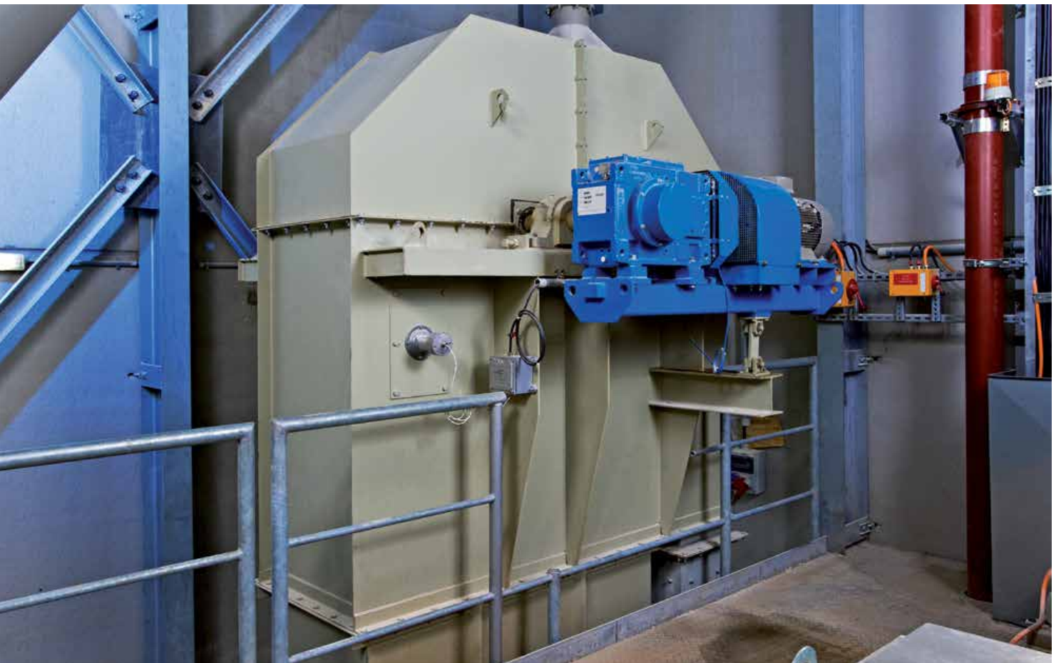
Bucket elevator head with single drive
